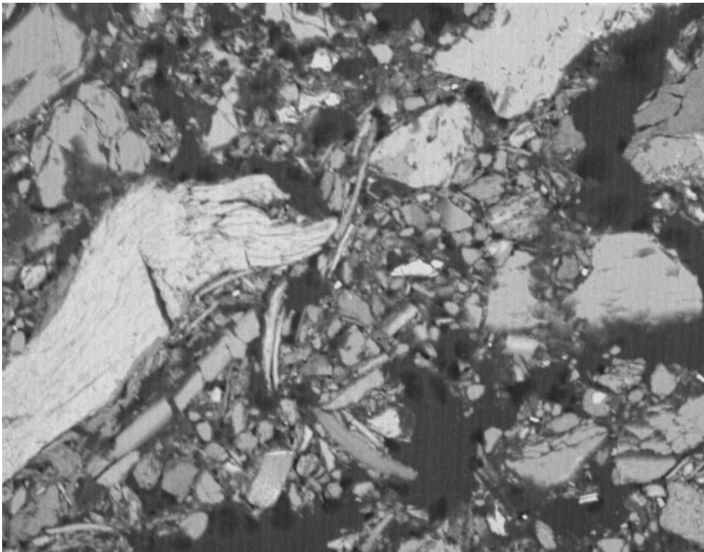
Figure 16. E-soil specimen exhibits a heterogeneous matrix with the upper image field width of 475 \mu\text{m} , and the lower 144 \mu\text{m} . The platy grains showing apparently good basal cleavage are probably a mica, or micaceous mineral.
