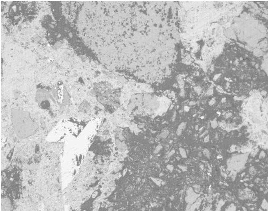
Figure 34. Another specimen from sample location I at 6 mm (upper) and 475 \mu\text{m} (lower) field width shows the heterogeneous phase distribution and microstructure distinctly different from that of the concretes.
