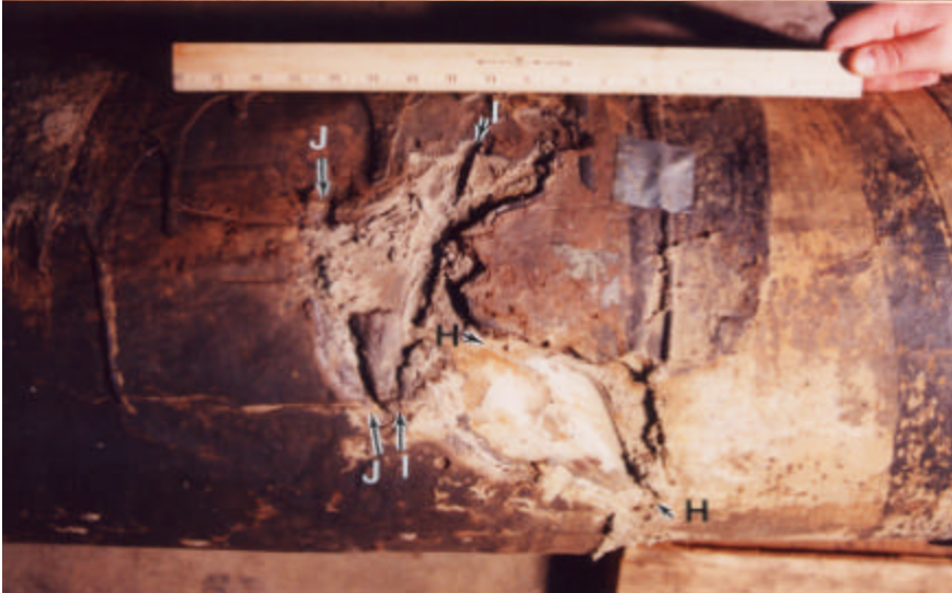
Figure 3. Close-up photograph of three gouge marks between arrows “H”, “I” and “J”. Samples removed from these gouge marks were labeled with the same letter designation, respectively.
