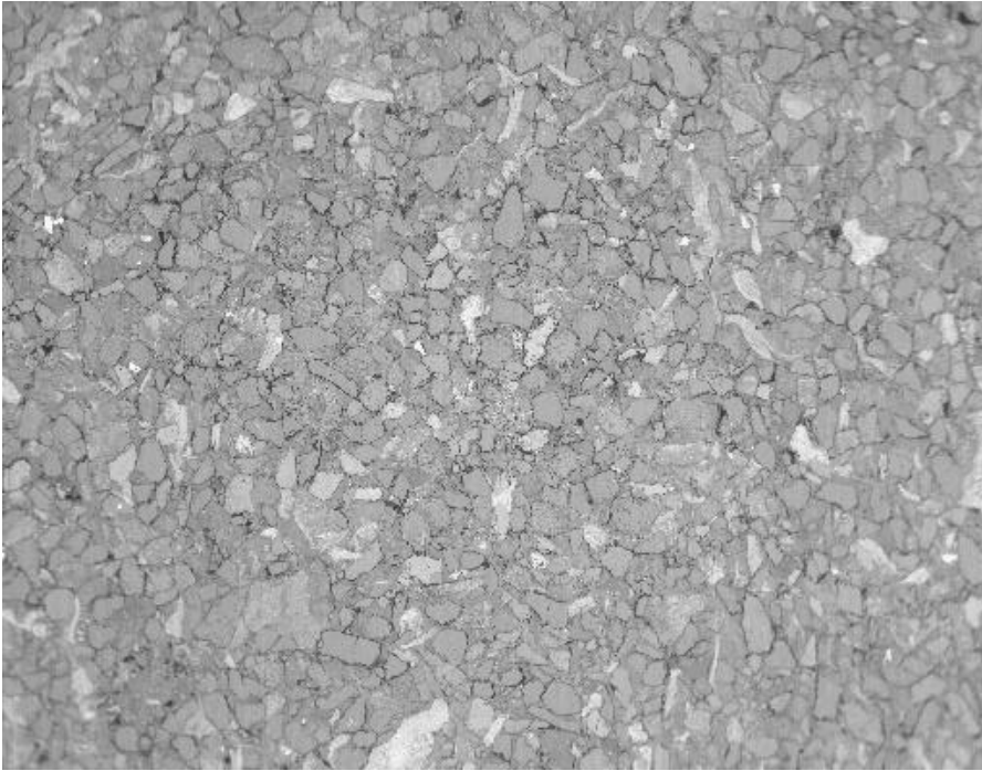
Figure 11. Scanning electron microscope backscattered electron image of an epoxy-impregnated, polished cross section of the back fill with uniform sand grading. Field Width: 4.9 mm
