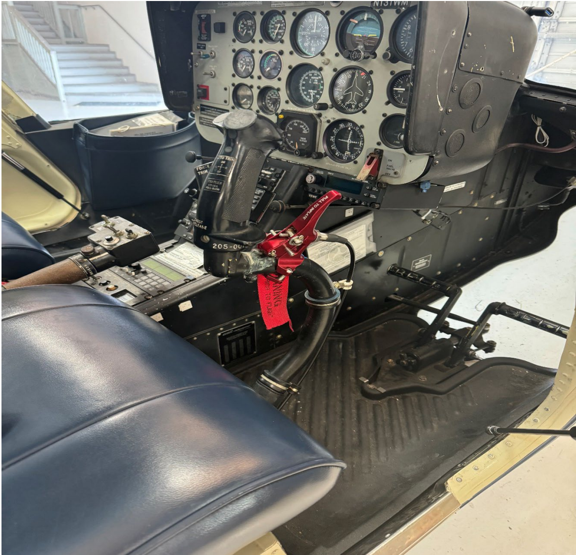
Photograph 3 Exemplar Cockpit Float Activation Lever (Red) Mounted on Cyclic Control (Courtesy of Westwind Helicopters)
