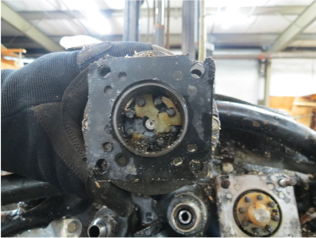
Photograph 2 – Aft side of vacuum pump with fragmented drive coupling.
