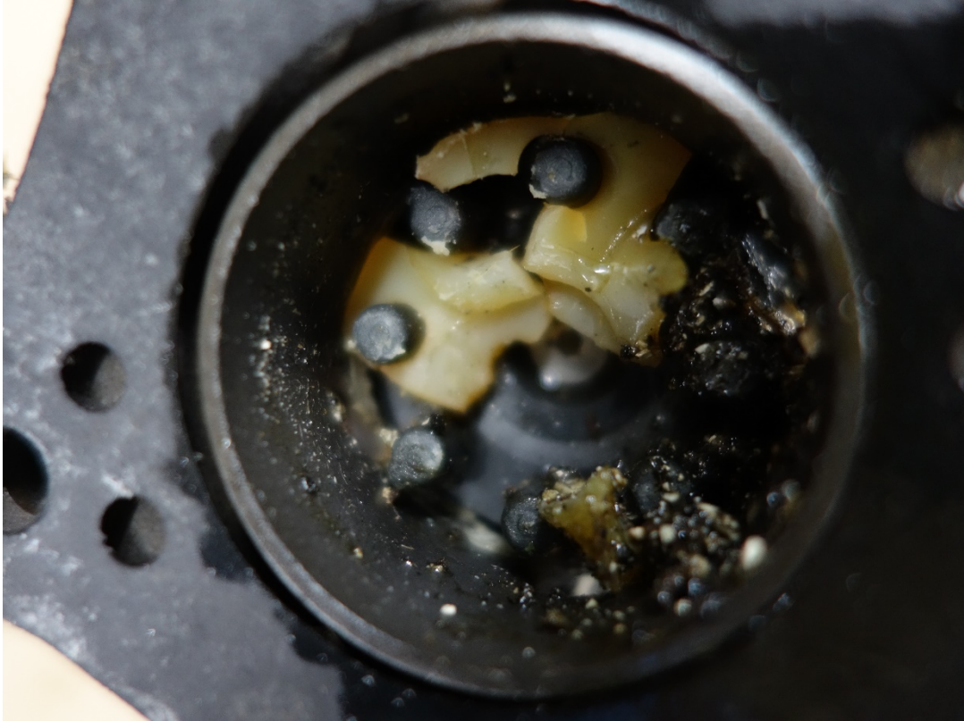
Photograph 6 – Vacuum pump - partial drive coupling.
