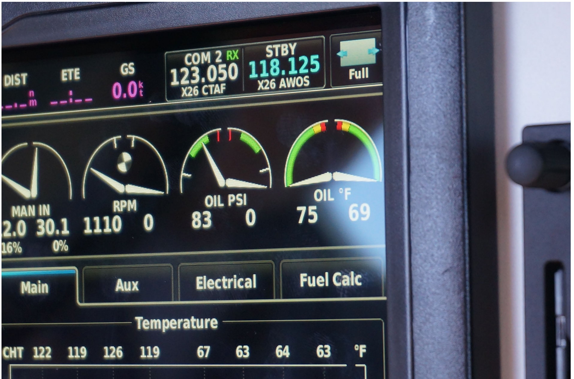
Photo 8 - Right Oil Pressure Sensor Test - Indicating Oil Pressure (Left "OIL PSI" Needle)
