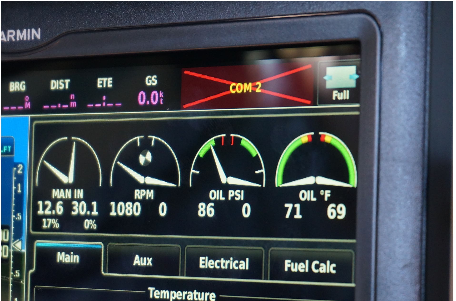
Photo 7 - Left Oil Pressure Sensor Test - Indicating Oil Pressure (Left "OIL PSI" Needle
