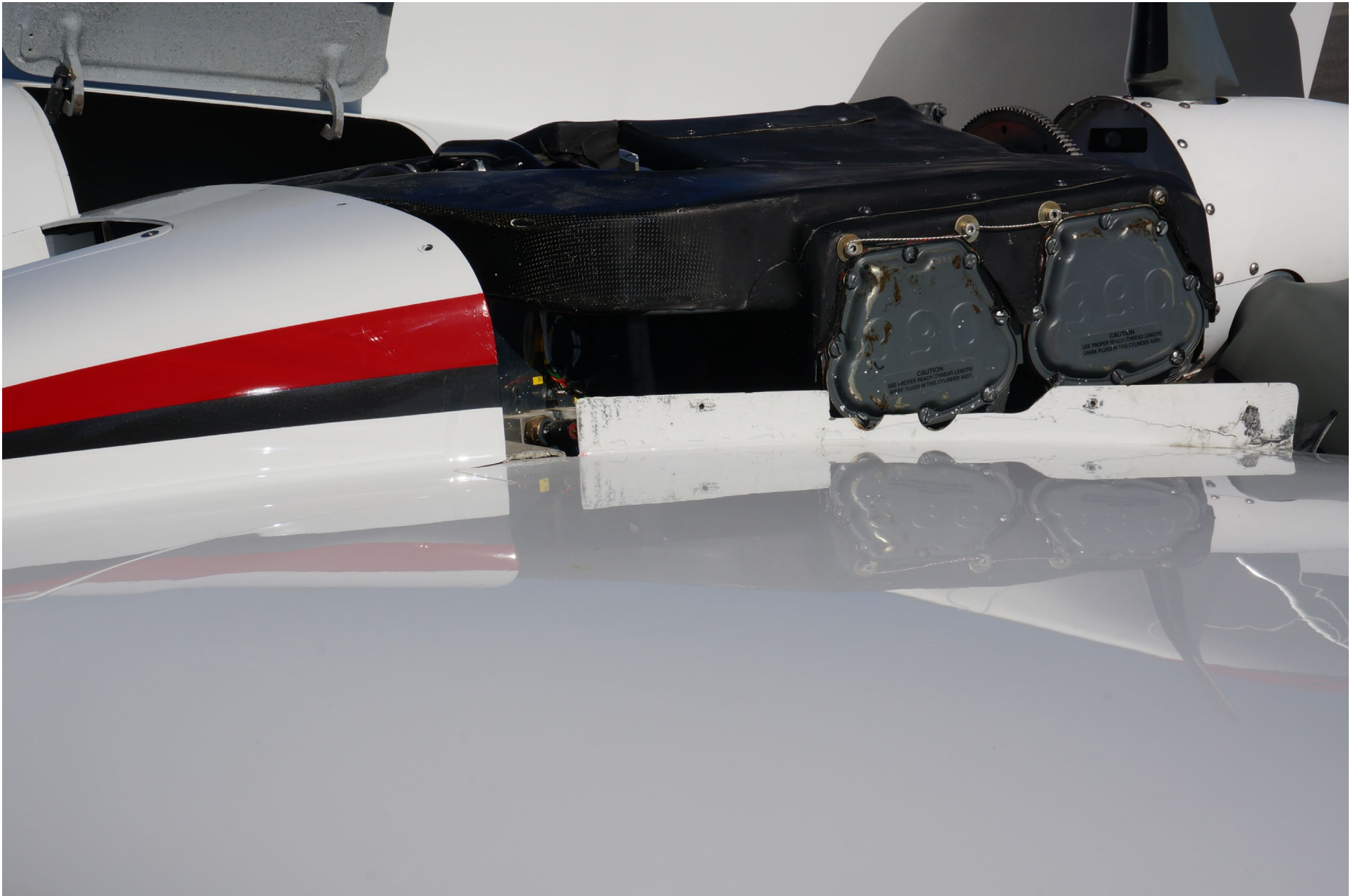
Photo 6 – Testing Location of Oil Pressure Sensors (Forward Left Engine Bay)
