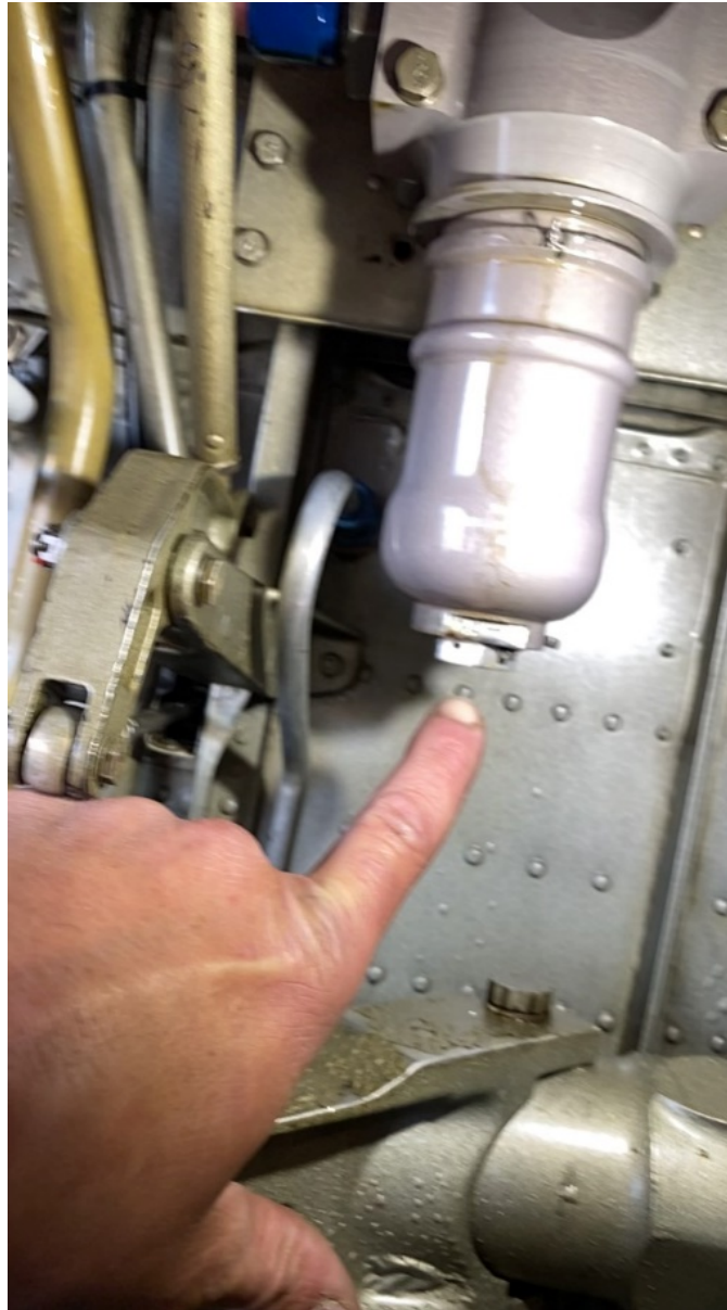
Figure 3: The airframe oil scavenge filter, with the red abnormal indicator stowed
