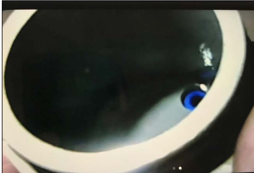
Photo 5: View of the engine driven fuel pump filter housing with remnants of fuel
