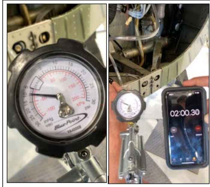
Figure 1: Photographs taken during the PC line pressure check
