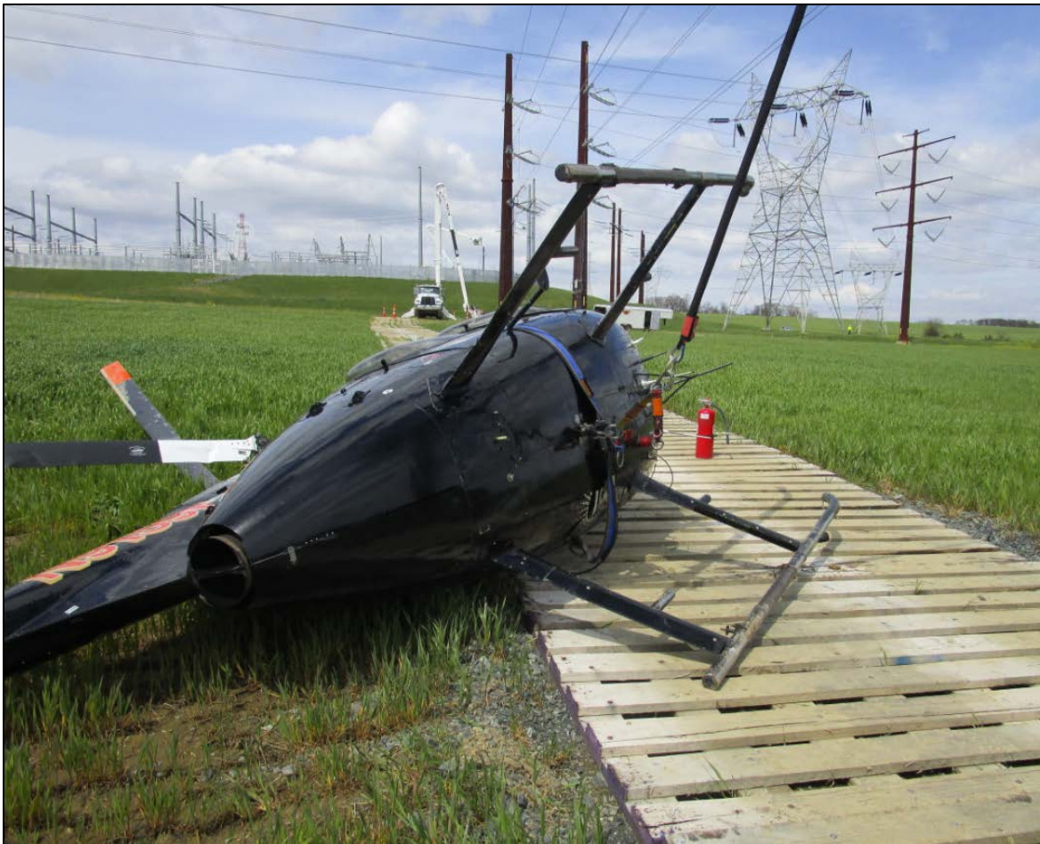
Figure 2: View of the helicopter with the belly band and the long line in view
