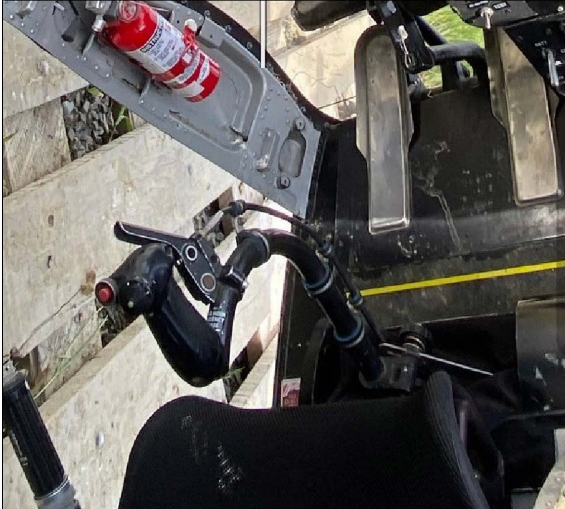
Figure 7: Additional view of the cyclic and the emergency release handle and red button
