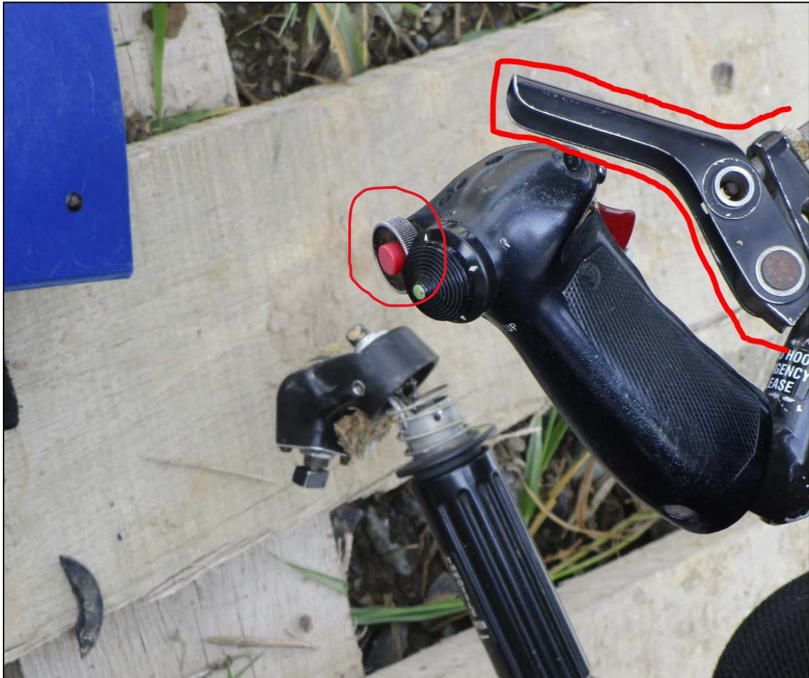
Figure 5: View of the two emergency release mechanisms for the long line main hook
