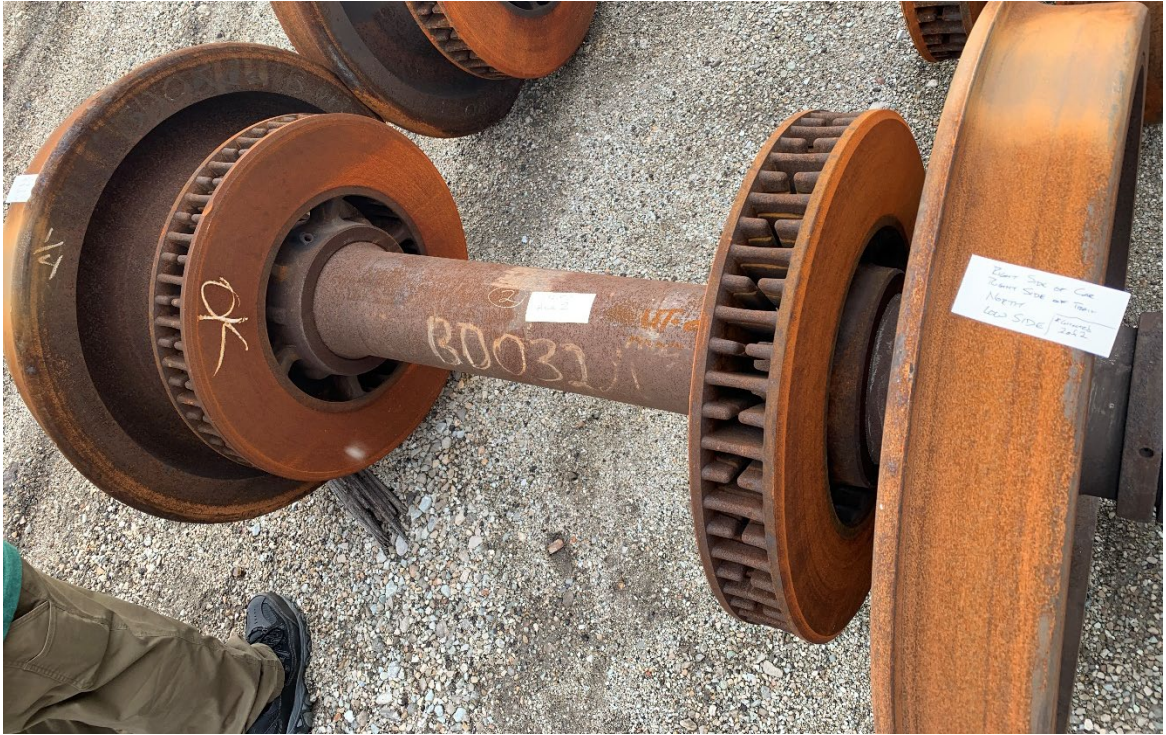
Figure 2. Car 32050 Wheelset No. 2 showing ID No. BDO3221 and tags placed by investigators at Beech Grove May 11, 2022
