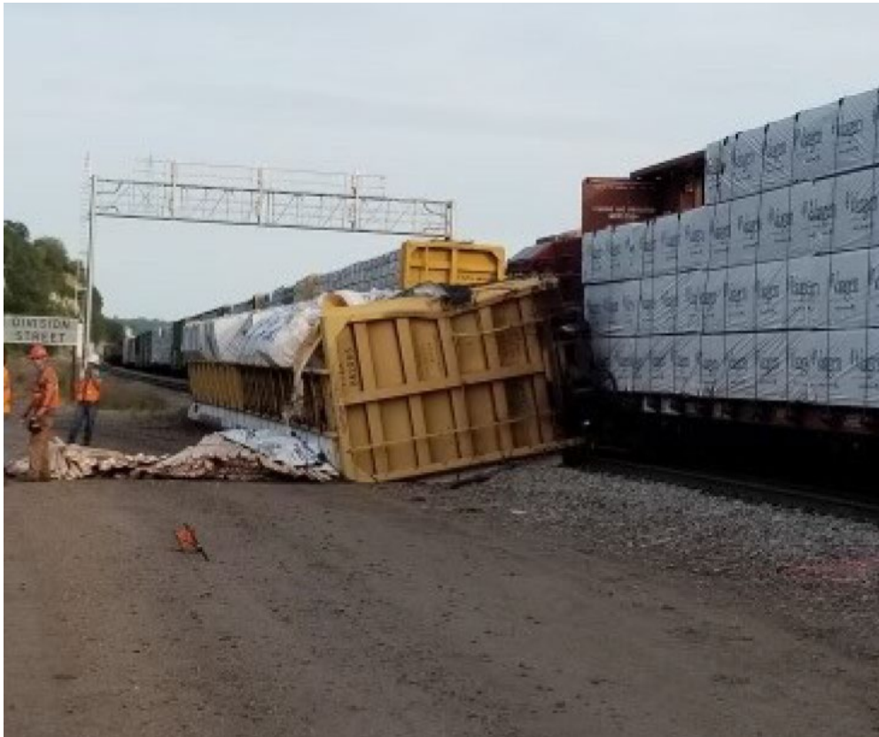
Figure 2 Photograph of the BNSF lumber car on its side after being struck and derailed. (Courtesy of FRA)
