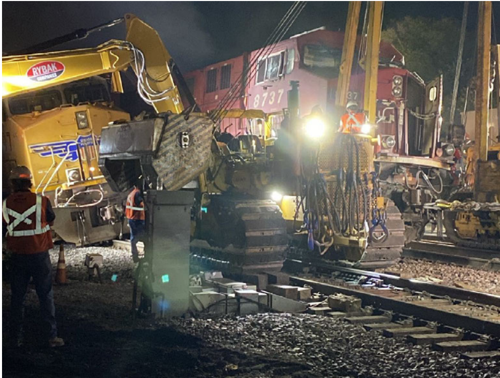
Figure 1 Photograph of the Union Pacific train (left) and the Canadian Pacific train (right) during rerailling operations. (Courtesy of FRA)
