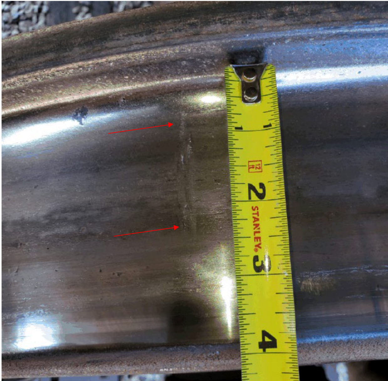
Figure 2 Photo of the witness mark on the right 3 wheel of car NATX 160112 (Photo by FRA)
