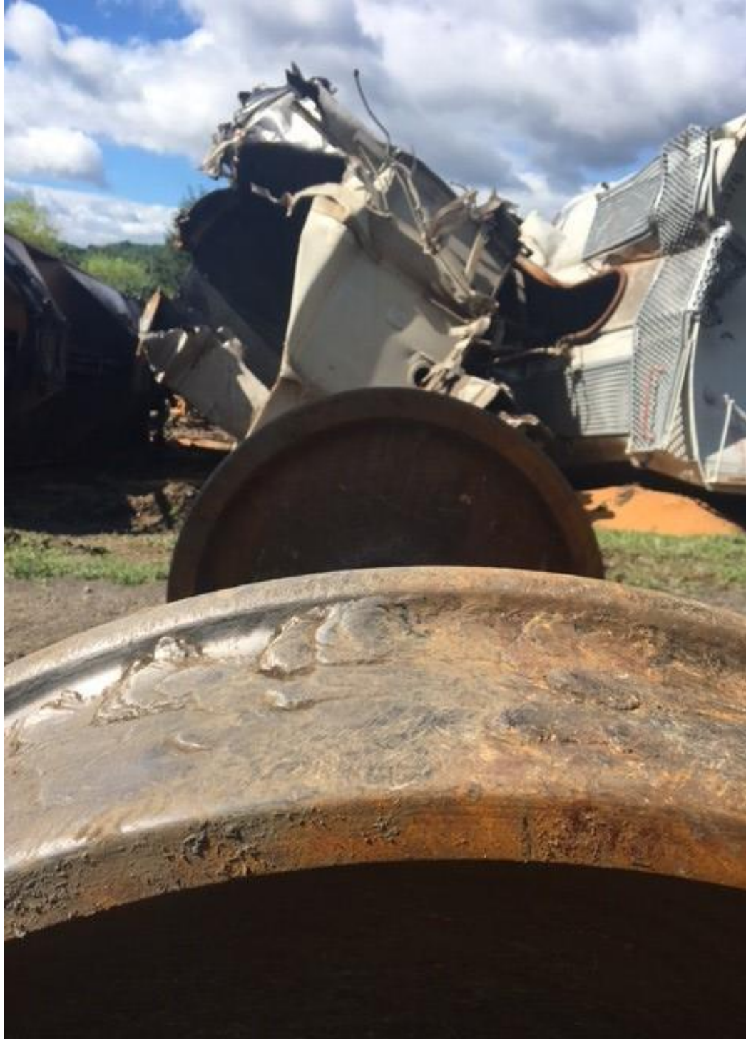
Figure 3. A close-up view of a wheel tread surface (from a wheel of the 35 th cars' #3-wheel set). Heavy metal build-up can be seen on the tread surface and in the throat of the wheel flange.
