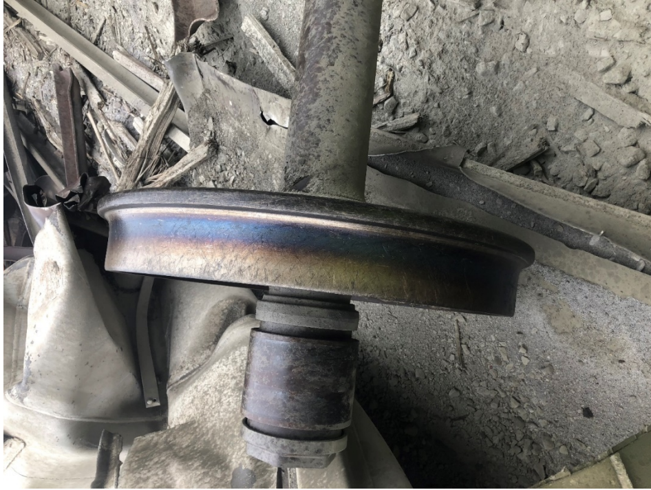
Figure 2 A wheel found toward the front end of the consist with bluing.
