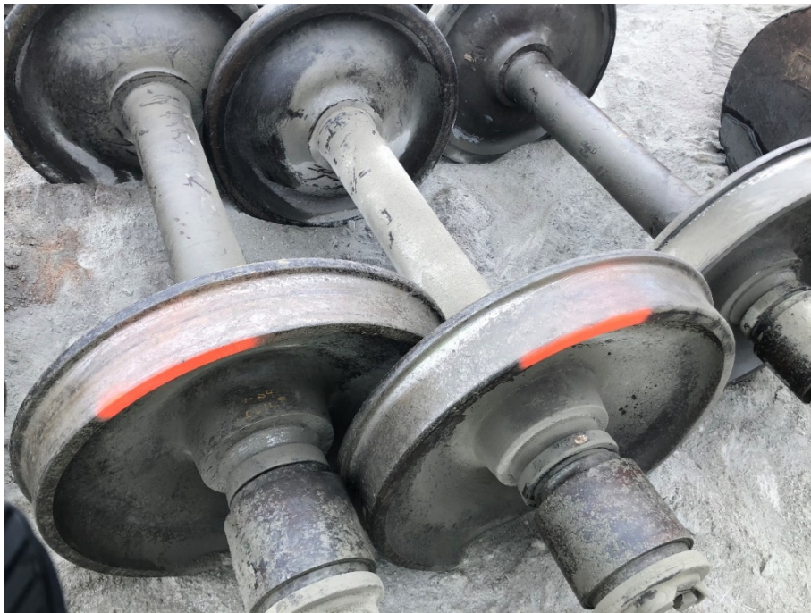
Figure 5 Marked wheels that show signs of overheating or sliding.
