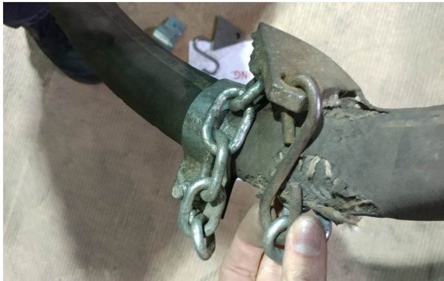
Figure 11Wear marks on the intermediate hose
