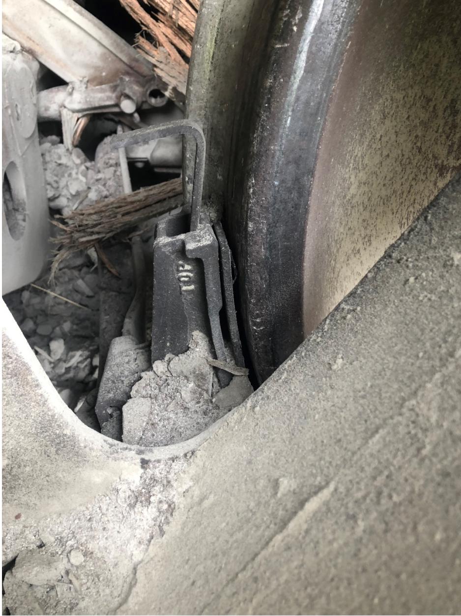
Figure 3 A worn brake shoe found towards the front of the consist.
