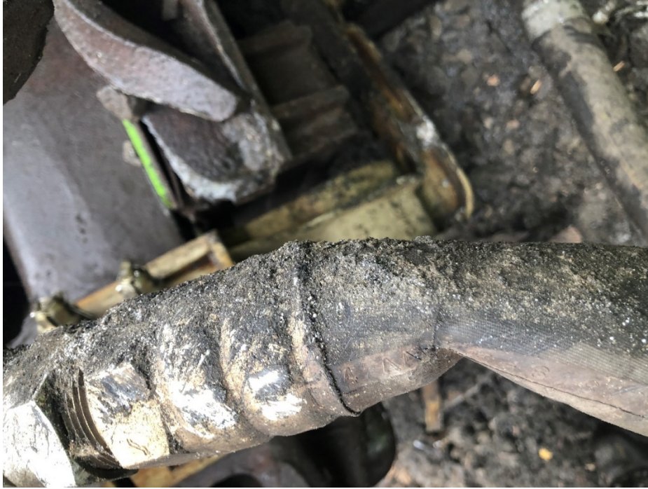
Figure 4 The "A" end intermediate air hose from car position 20.
