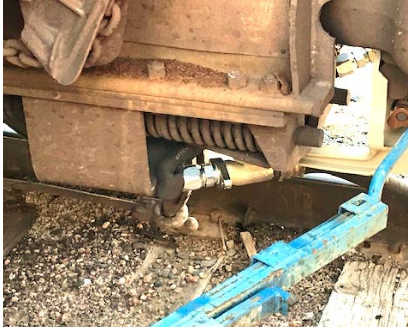
Figure 7 Kinked intermediate air hose after misapplication.
