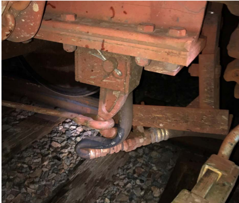
Figure 6 Kinked air hose on car west of Cheyenne, WY.
