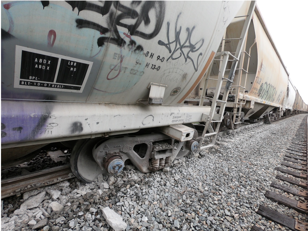
Figure 1. LEHX 1008-first car to derail.
