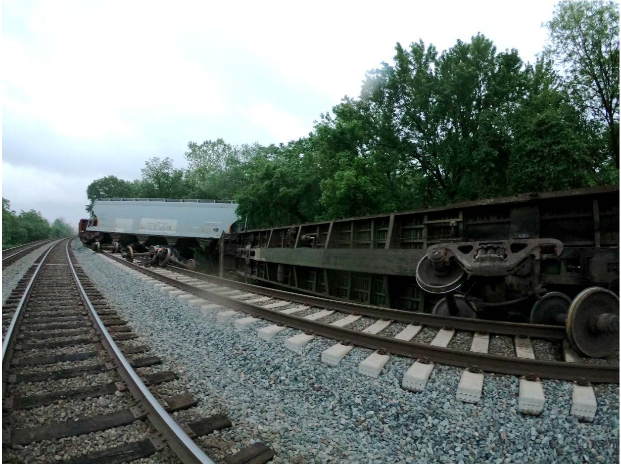
Figure 5. Photograph of secondary derailment.
