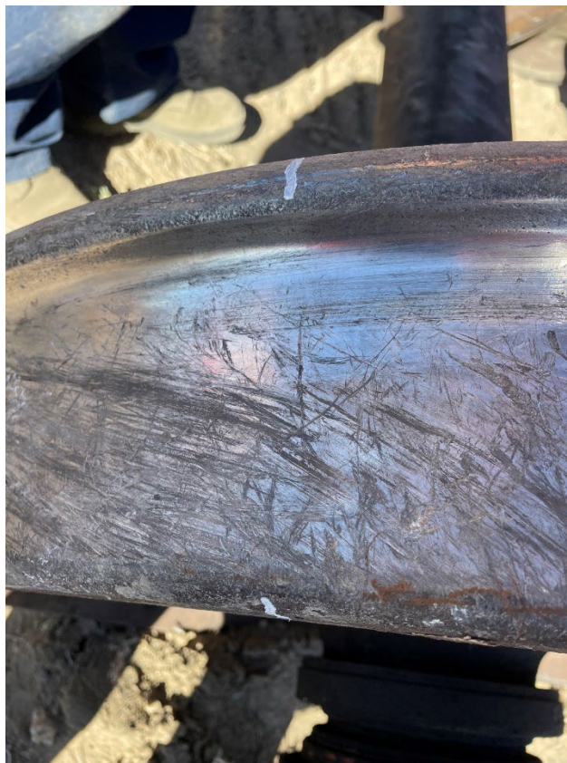
Figure 2 - Wheel from one of the railcars that passed over the broken rail with rail impact indentation.
