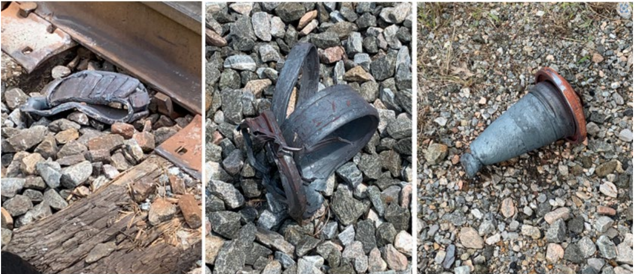
Figure 1: Photographs of Car CR 507499 - failed (burned off) journal bearing components
