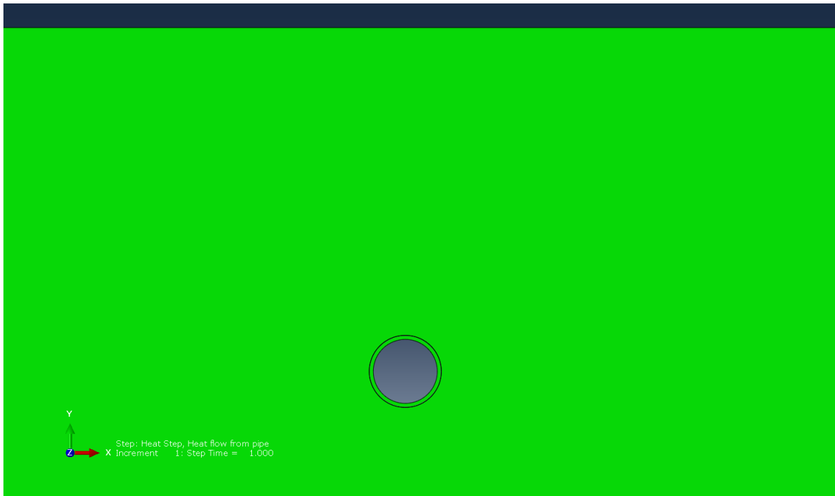
Figure 1. Overview of model used to calculate the steady-state temperature distribution around the buried pipe: a) low mag and b) high mag.
