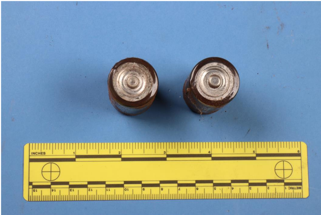
Figure 5: Transducer batteries positive pole.
