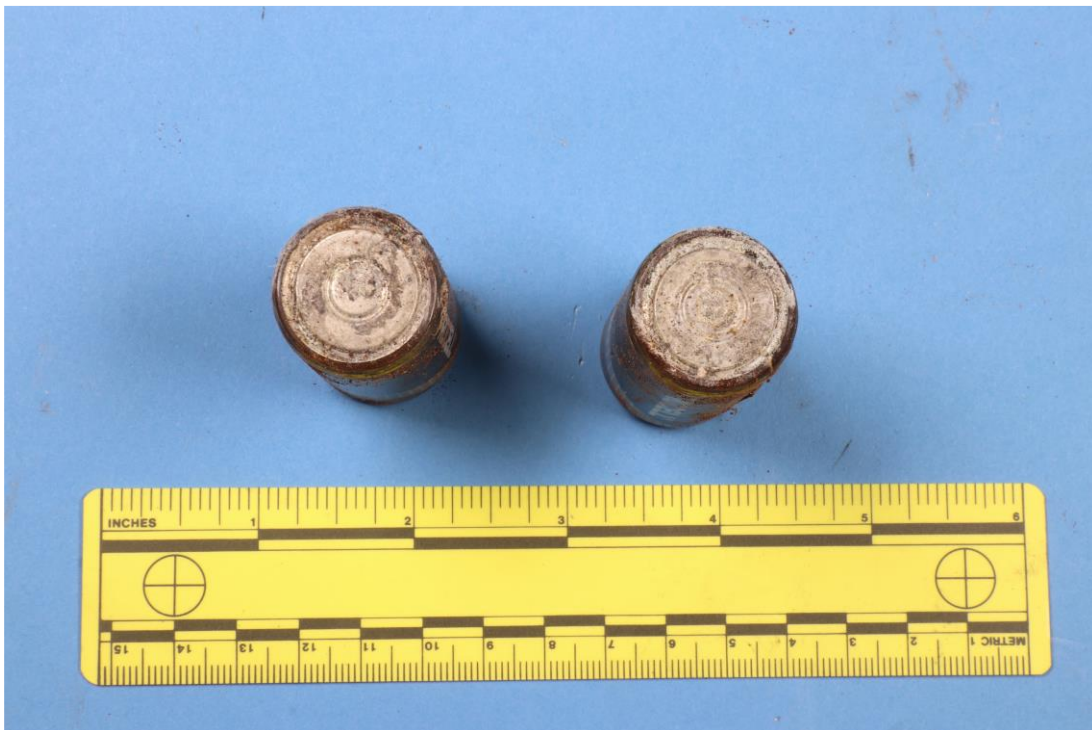
Figure 4: Transducer batteries negative pole.
