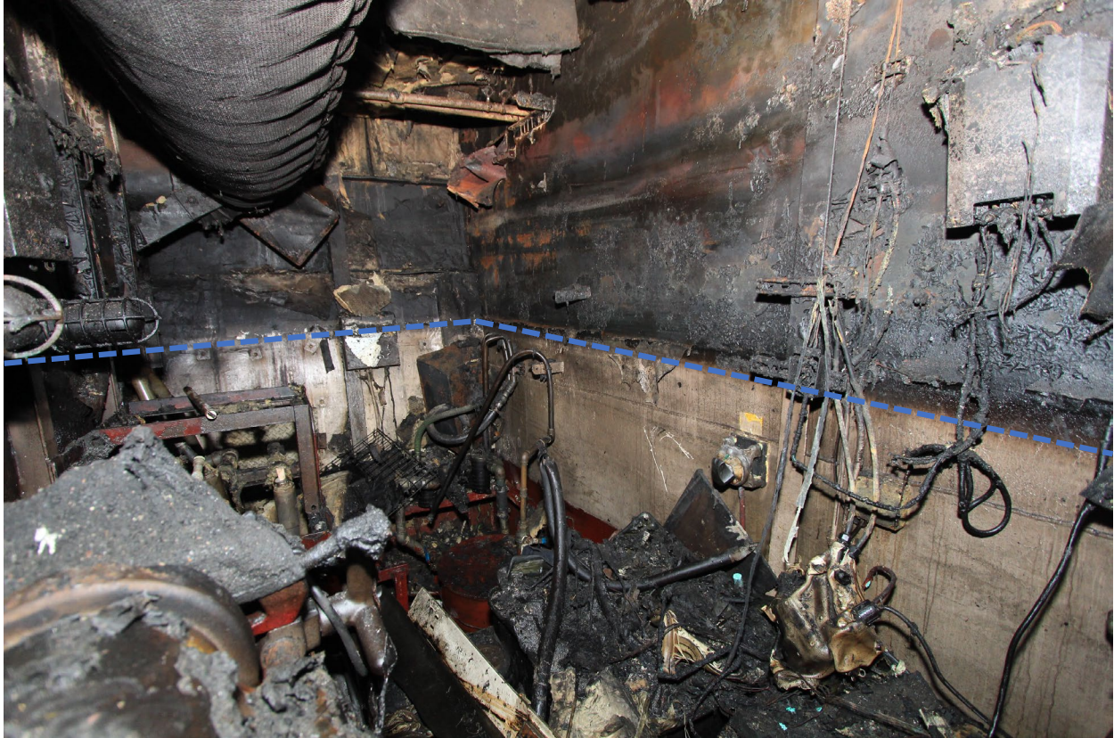
Figure 18. Alcove forward of port main engine exhibiting demarcation between thermally damaged and undamaged area.
