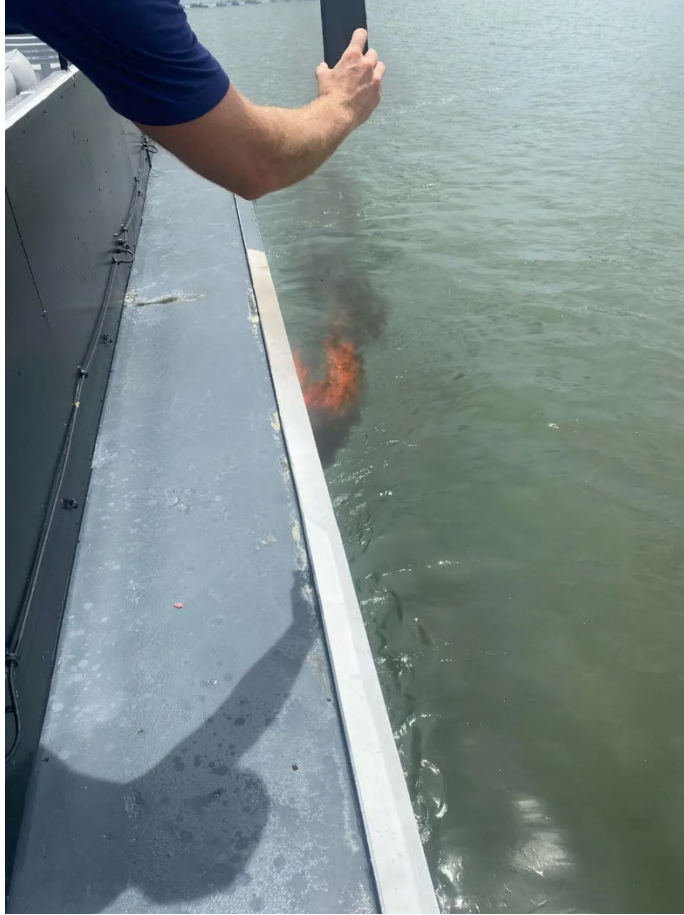
Figure 15. Photo of smoke and flame exiting port side engine room vent. (Source: Passenger Jason Sleeth).
