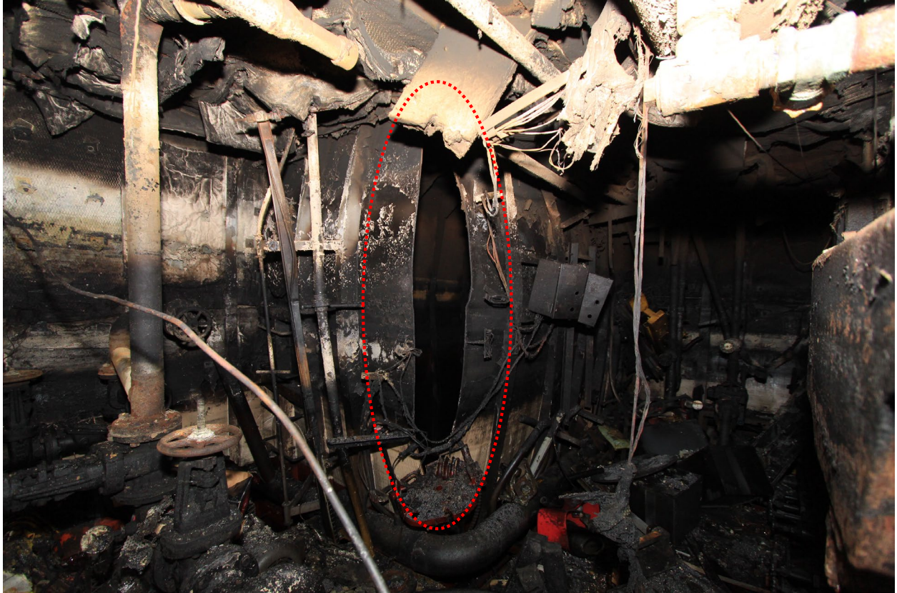
Figure 26. Starboard fuel tank fracture.
