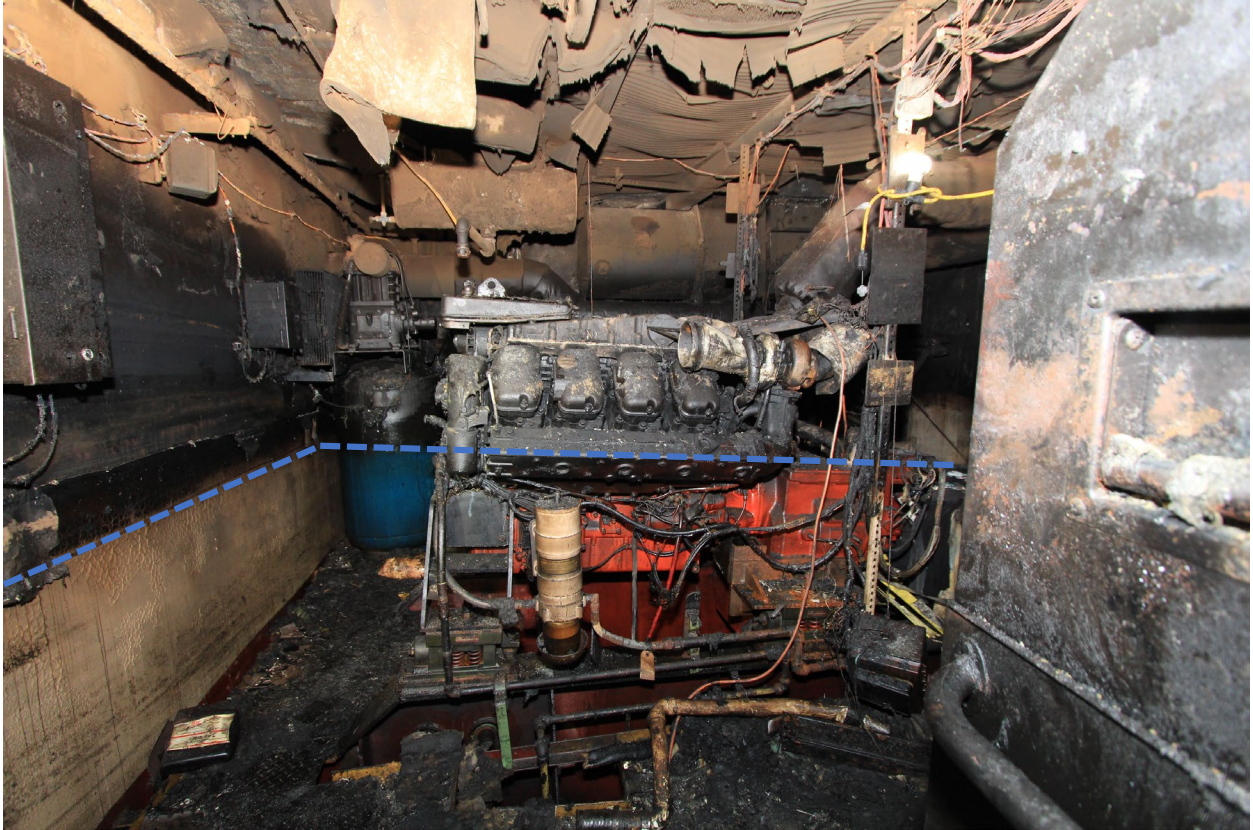
Figure 19. Starboard main engine exhibiting demarcation between thermally damaged and undamaged area.
