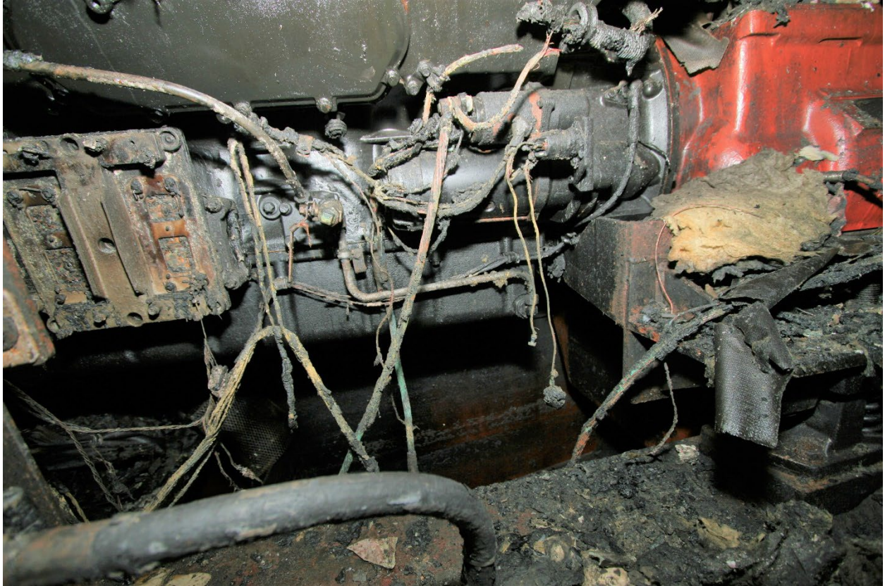
Figure 24. Gear box aft of port main engine with intact paint.
