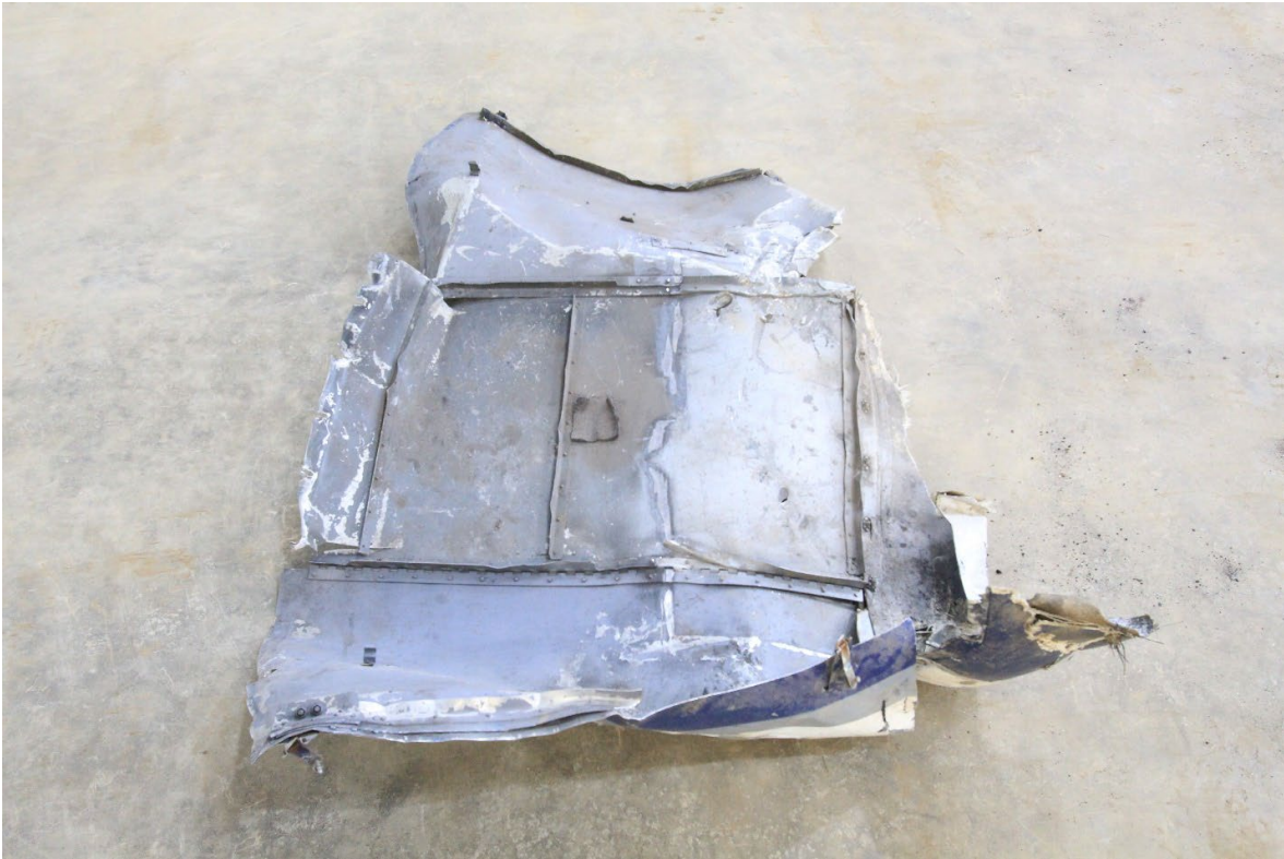
Figure 9. Interior surface of the portion of engine cowling.
