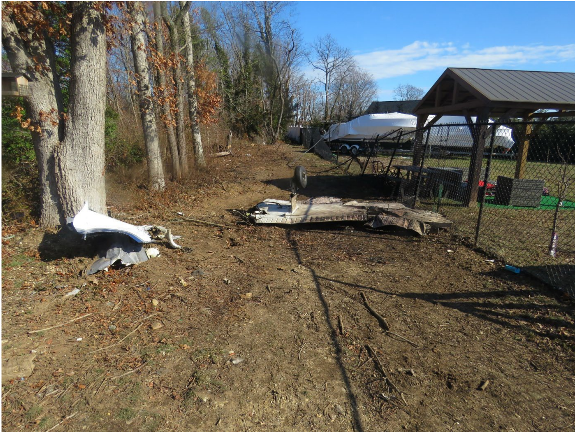
Figure 2. A portion of left wing with main landing gear attached. A portion of the engine cowling can be seen at the base of a tree.
