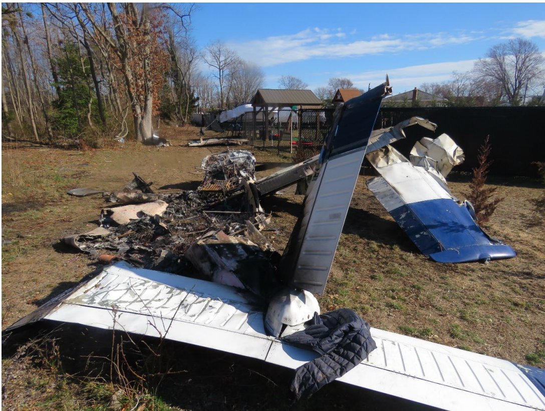
Figure 1. Resting position of the aircraft at the accident site. The aircraft spun around and was facing opposite the direction of travel.
