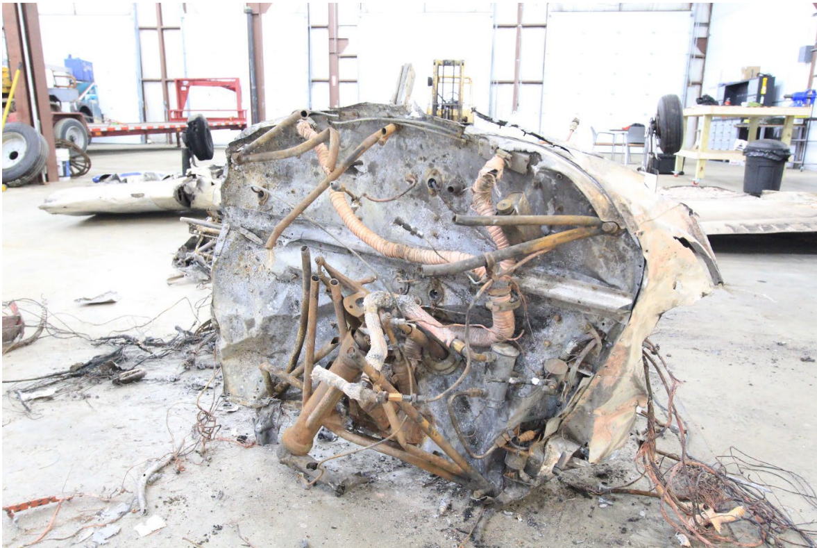
Figure 11. Engine side of the firewall.
