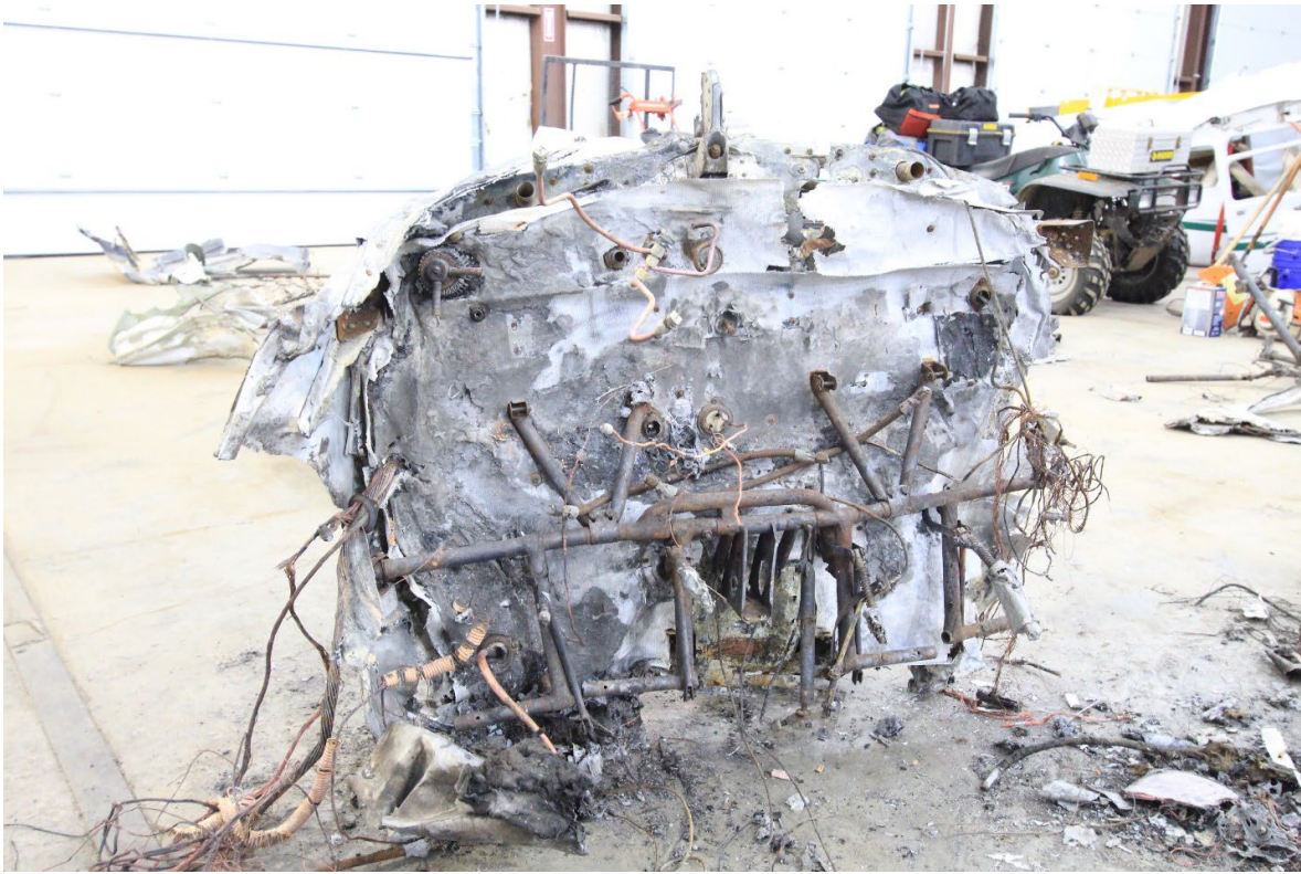
Figure 12. Cockpit side of the firewall.
