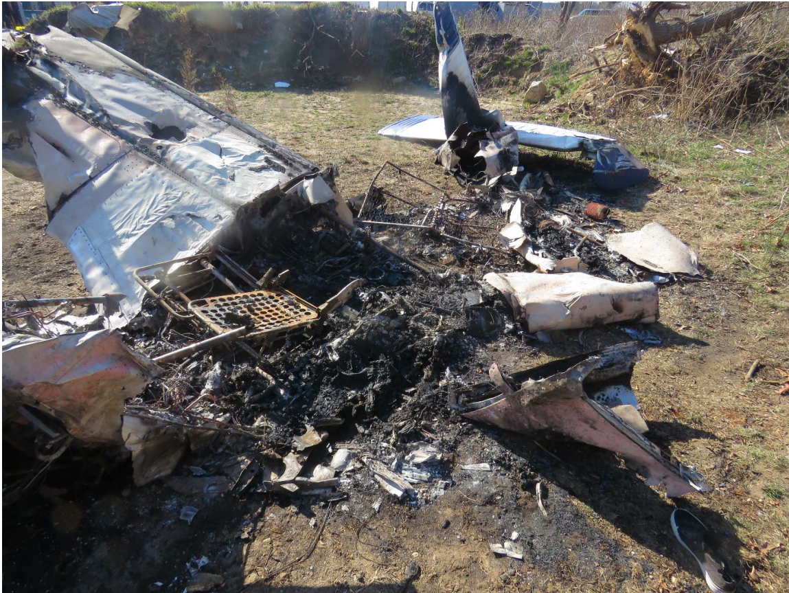
Figure 3. Remaining portions of the aircraft fuselage.
