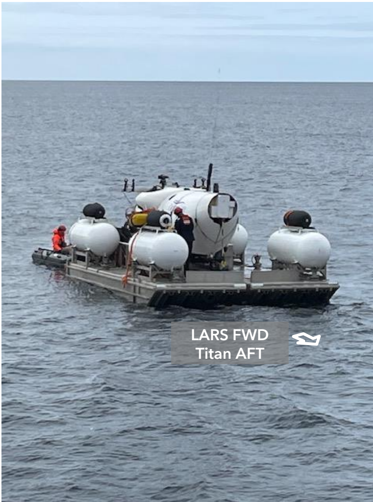
Figure 40. Images of tipping/upset events during 2023 expedition (Source: Steven Taragel): a) Post recovery after the forward end of the LARS (aft end of Titan) tipped downward. The tail cone separated as a result of the mishap; b) tipping event with the aft starboard corner of the LARS tipped downward; and
