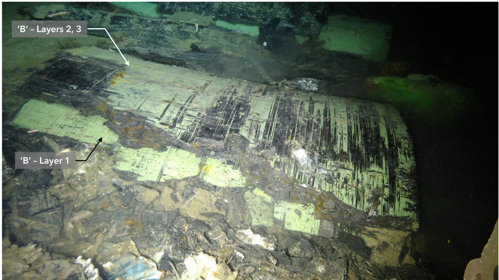
Figure 20. View of piece 'B' after removal of layers 4 and 5. The fracture along the CCW edge was irregular.
