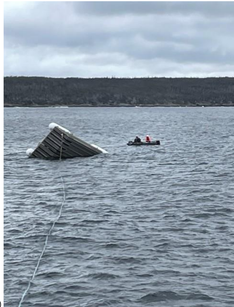
Figure 40. Images of tipping/upset events during 2023 expedition (Source: Steven Taragel): a) Post recovery after the forward end of the LARS (aft end of Titan) tipped downward. The tail cone separated as a result of the mishap; b) tipping event with the aft starboard corner of the LARS tipped downward; and
