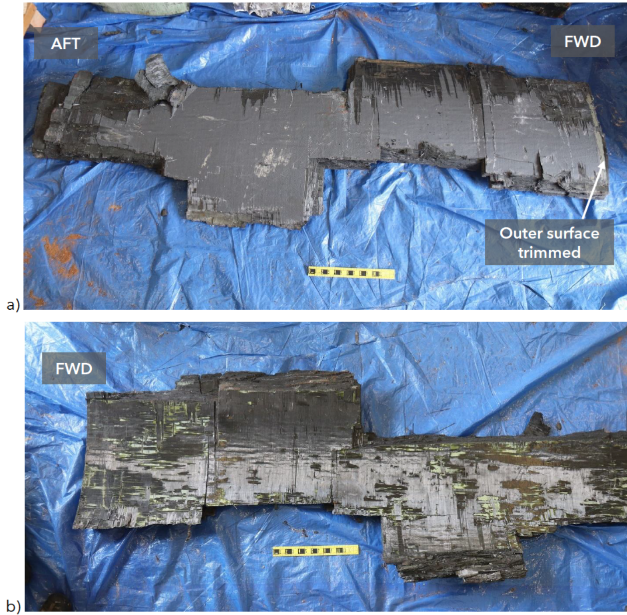
Figure 48. Images of large layer 4 and 5 hull piece: a) outer surface and b) inner surface.
