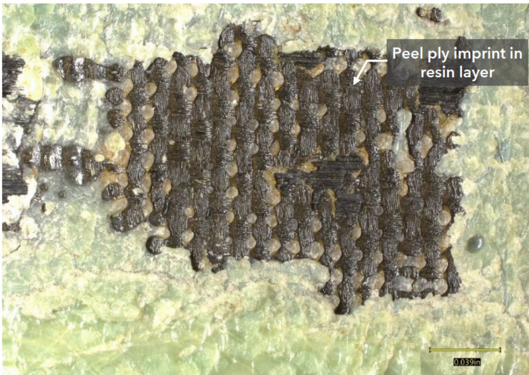
Figure 9. Images of layer 1 surface: a) region with all the components of the layer interface with labels; b) void in adhesive. Underlying resin with a peel ply imprint is exposed.
