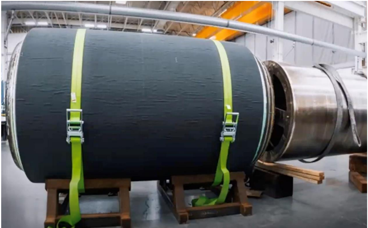
Figure 49. Images showing waviness on the outer surface of the hull: Upper image: retrieved hull piece. Lower image: Rough hull post-curing with mandrel removed.
