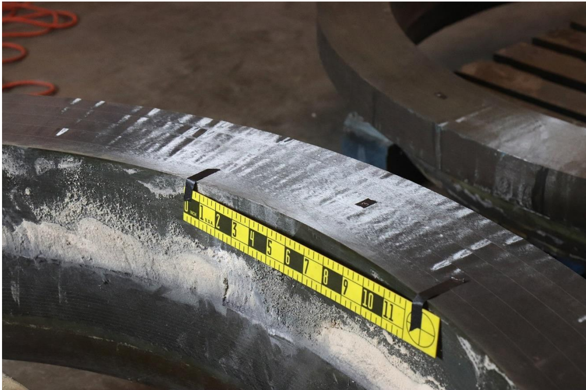
Figure 28. Images of the trimmed end faces under oblique lighting showing wrinkles and waviness in the carbon fiber orientation. Local variations in fiber orientation result in the observed light/dark brightness variations; a) trimmed end 'A' and b) trimmed end 'B'.
