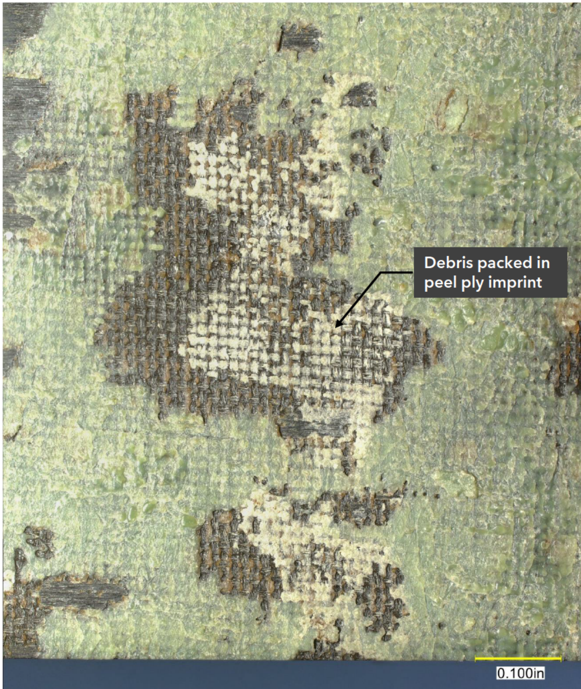
a) Figure 22. a) Void in adhesive layer prior to cleaning with debris packed into the peel ply imprint and
