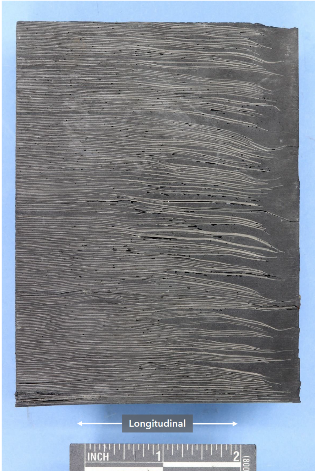
Figure 38 (cont.). b) longitudinal cross section of the trimmed end piece from the first full scale Titan hull.
