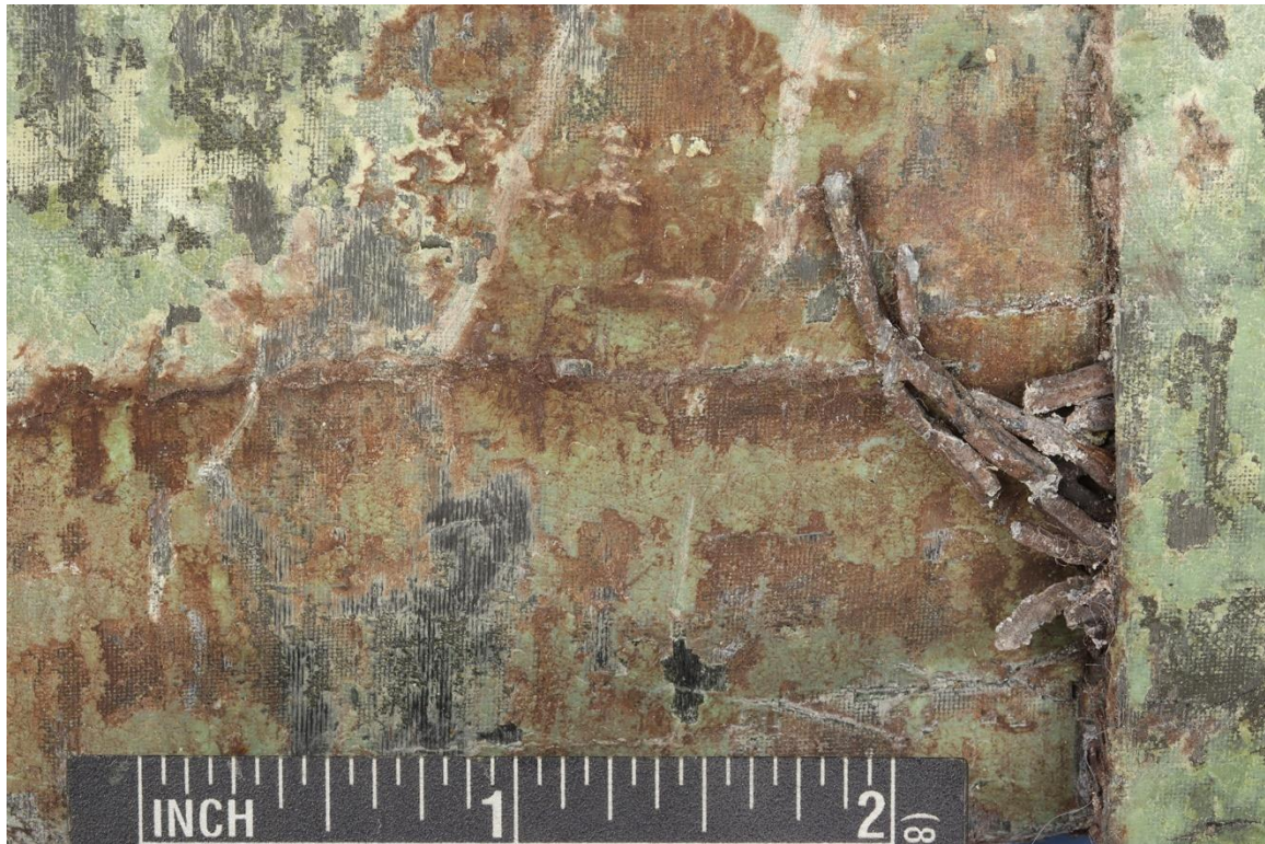
Figure 24. Contact marks on the left side: a) image showing both contact marks and b) higher magnification image of the forward mark showing the embedded object, identified as lead.
