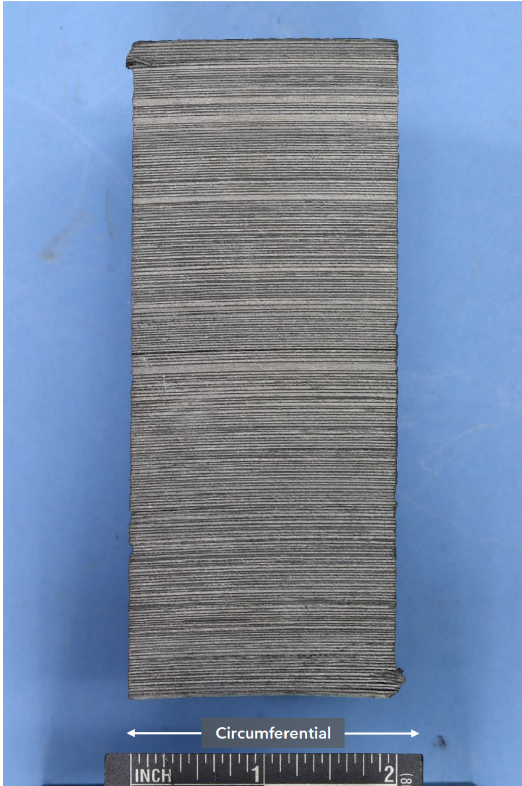
Figure 38. a) Circumferential cross section of the trimmed end piece from the first full scale Titan hull and
