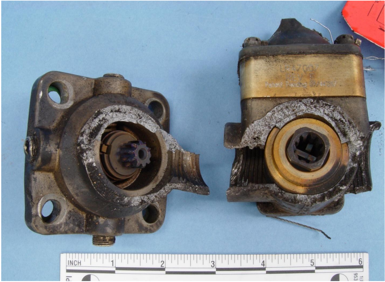
Figure 16: Low-pressure engine-driven fuel pump as received.
