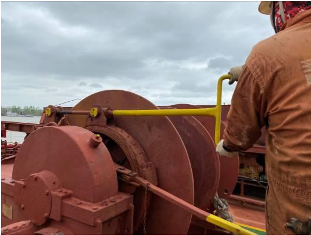
27. Forward Midship mooring winch break test.
