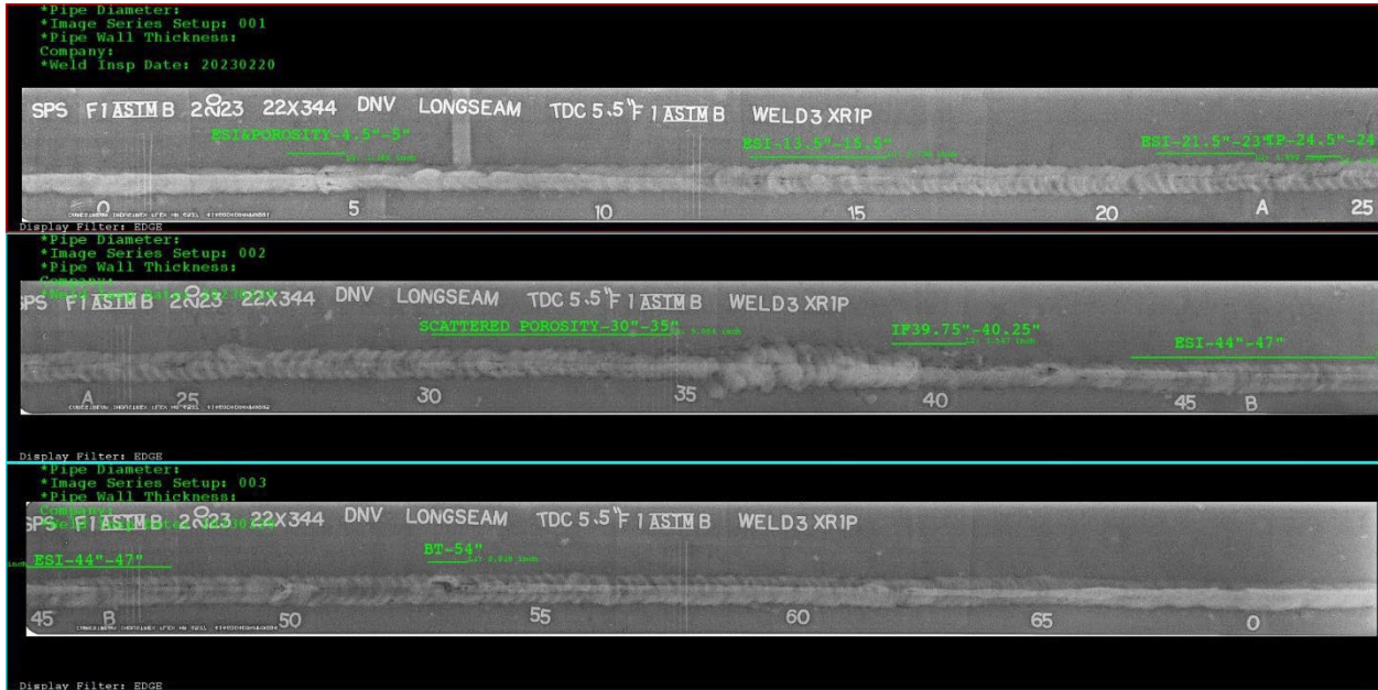
Figure 3: RT image of intact girth weld.
