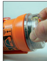
Reinstall lid- tighten without tools
