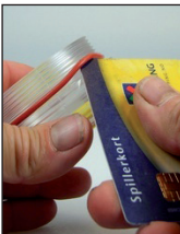
Remove old O-ring using a Credit Card
