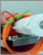
Install the new battery. Make sure the cable is within the guide
