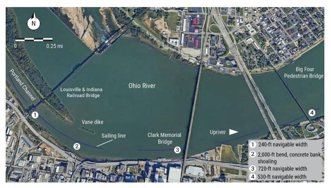
**Figure 7.** Navigational considerations for a vessel transiting upriver on the portion of the Ohio River between the Louisville and Indiana Railroad Bridge and the Big Four Pedestrian Bridge. (Background source: Google Earth)
