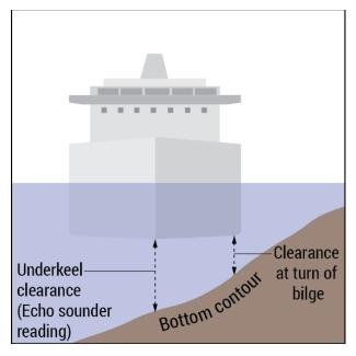
**Figure 10.** Exemplar of relative difference in hull clearances along a sloped bank/shoal. (Illustration does not reflect actual contour or vessel in this casualty.)
