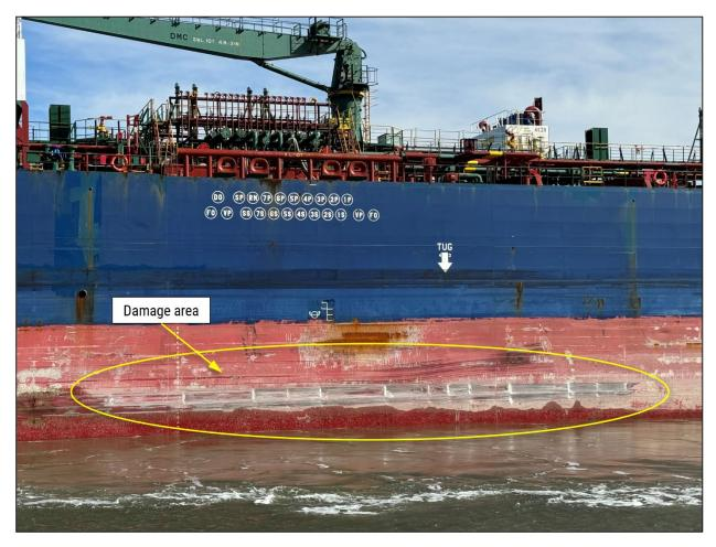
**Figure 5.** Hafnia Amessi starboard side after the contact, showing inset plating and scraped paint within circled area. (Background source: Coast Guard)
