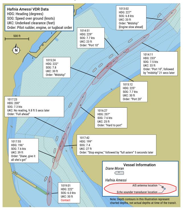
**Figure 4.** Hafnia Amessi automatic identification system (AIS) trackline. (Background source: NOAA ENC US5SC1LO as viewed on Made Smart)
