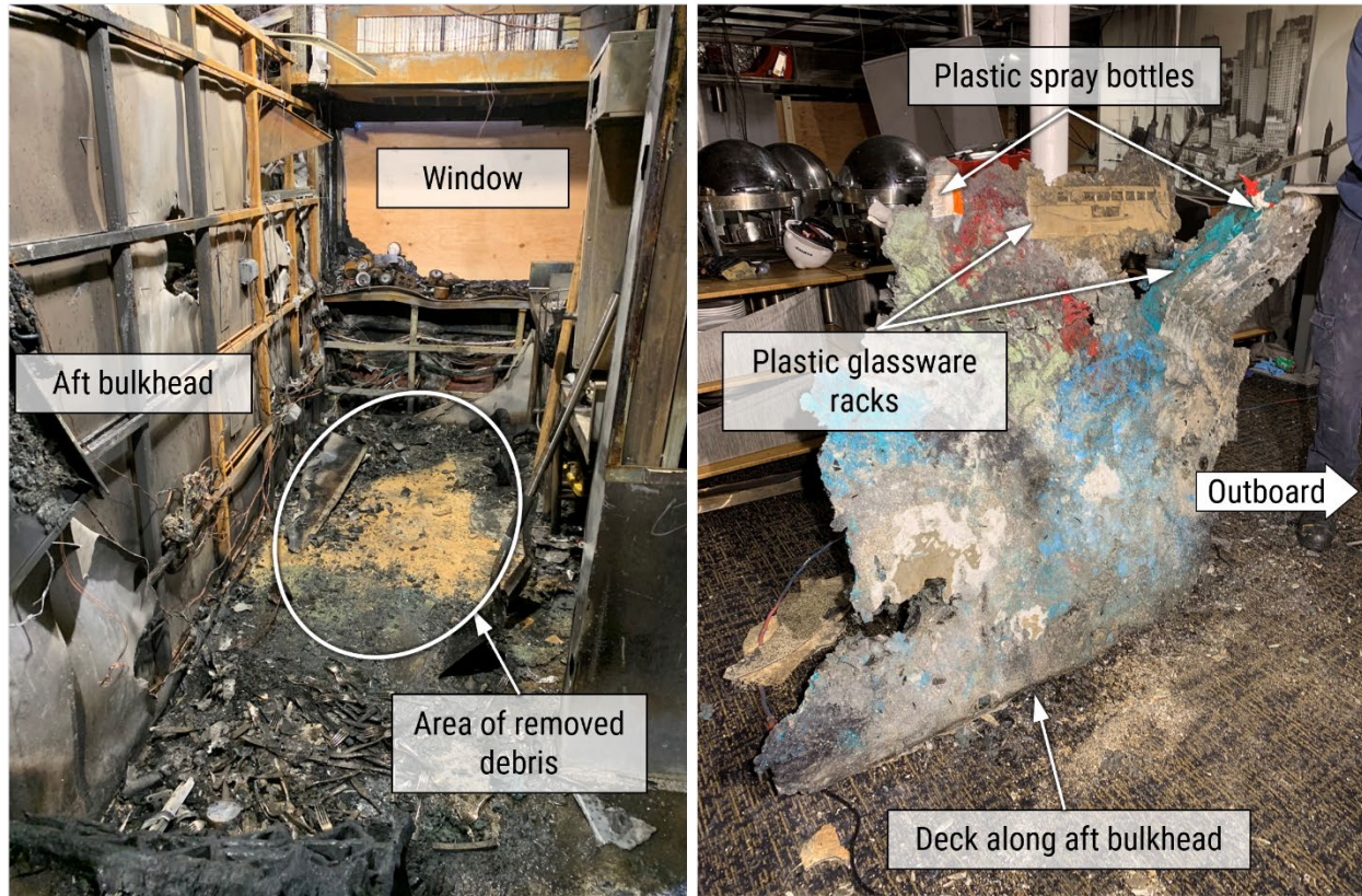
Figure 15. Left to right: Location of the melted mass of debris—comprising the remains of the plastic glassware rolling carts—removed from the deck 1 wait station on Spirit of Boston after the fire. Bottom of the melted mass of debris from the wait station after flooring material was removed. (Figure 8 shows the deck 1 wait station layout before the fire.)
