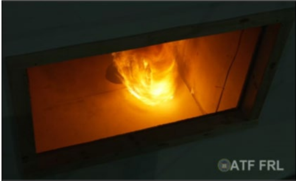
Figure 18. Screenshot of video looking through window of ATF test structure in replicated deck 1 wait station showing flame vectoring and liquified plastic pool (to left of flames) in the area where the plastic glassware rolling cart was located. (Source: ATF)
