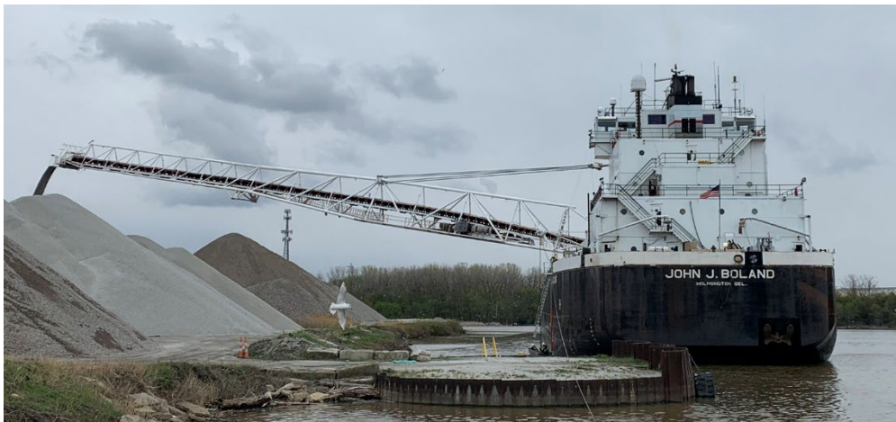
Figure 1. John J Boland discharging cargo from its port side using its self-unloading boom in Lorain, Ohio, after the grounding.
