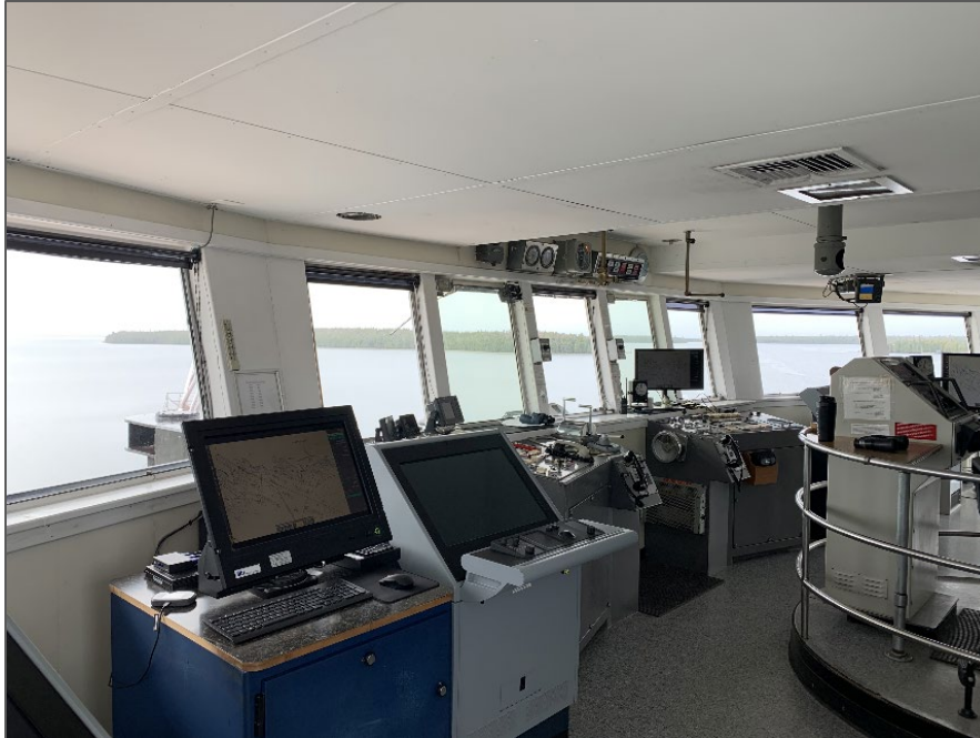
Figure 6. American Mariner's bridge and centerline conning station. (Source: Coast Guard)
