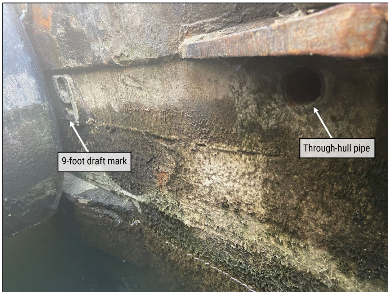
Figure 7. Joanne Marie through-hull pipe for the cofferdam pumps' overboard discharge on the port quarter with 9-foot draft mark shown postcasualty. (Background source: Coast Guard)
