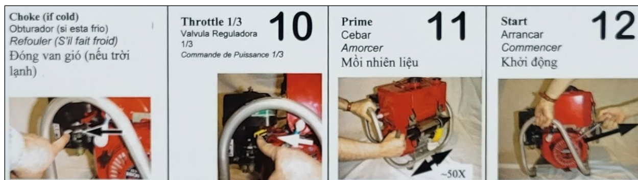
Figure 6. An excerpt of the instructions included with the P6 pump like the one sent to the Captain Alex . The instructions show the priming sequence and include steps written in four languages: English, Spanish, French, and Vietnamese (the native language of the Captain Alex crew). (Source: Coast Guard)
