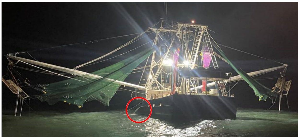
Figure 5. The Captain Alex with discharge stream from bilge system (indicated by red circle) at 0317, just after CG 45630 arrived on scene. (Source: Coast Guard)
