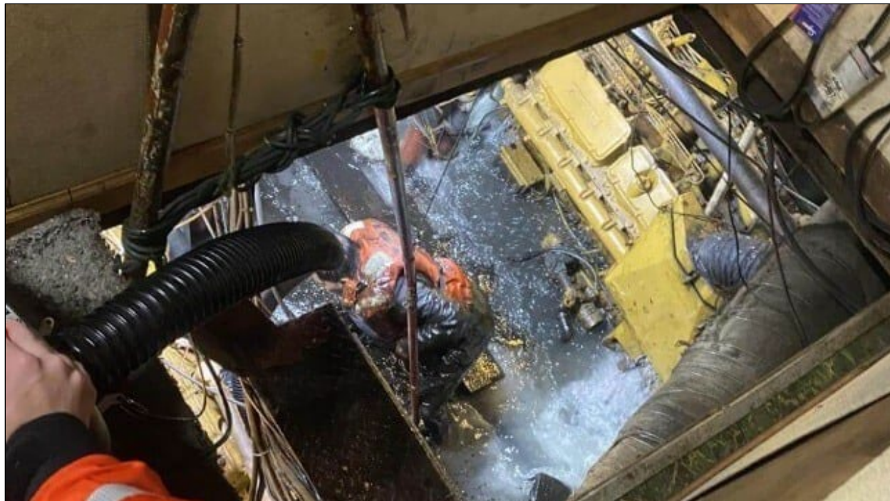
Figure 4. Looking down into the engine room of the Captain Alex at 0326, with the water midway up the starboard main engine and the captain of the vessel on the stairs. The suction hose to the portable dewatering pump (on deck) is on the left. (Source: Coast Guard)
