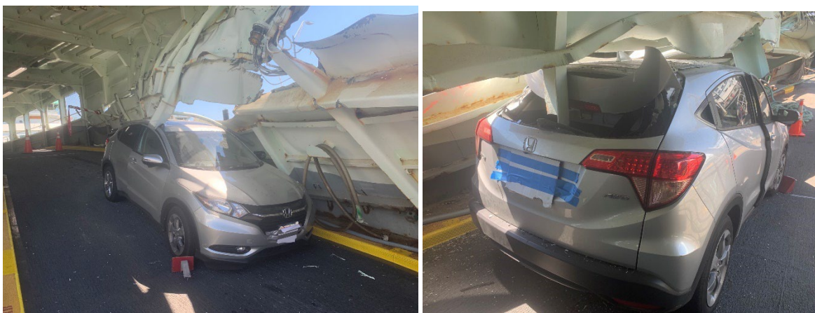
Figure 9. Damage to the front ( left ) and back ( right ) of the vehicle impacted by the vessel structure.
