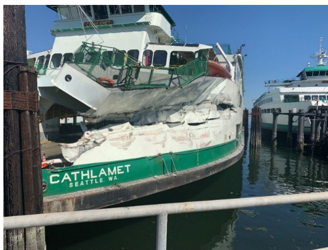
Figure 8. The damaged Cathlamet after the contact with the dolphin.
