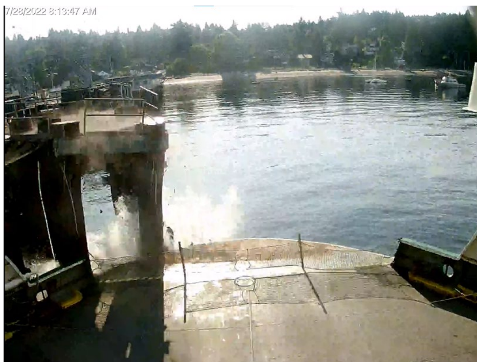
Figure 5. Still image from forward-looking camera footage on board the Cathlamet at the time the ferry's port bow struck the dolphin. (Source: Washington State Patrol)
