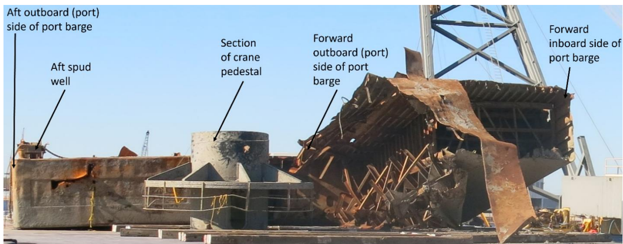
Figure 7. The two sections of barge GD 962 (the Ambition's port barge) after recovery from the Gulf of Mexico.
