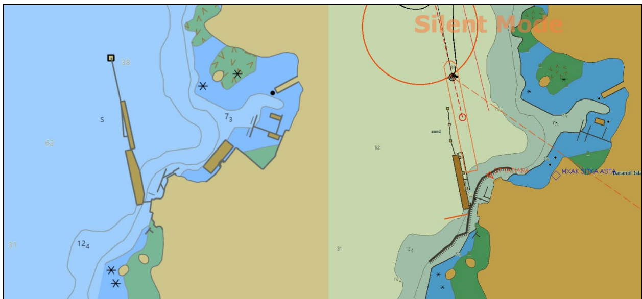
Figure 7. ENC updated postcasualty ( left ) and as seen on Radiance of the Seas ’s ECDIS ( right ) with the ship’s outline after mooring shown in orange. (Sources: NOAA [ left ] and Royal Caribbean Cruise Lines [ right ])
