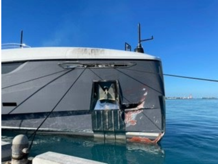
Figure 6. Damage to Utopia IV 's bow. (Source: Coast Guard)
