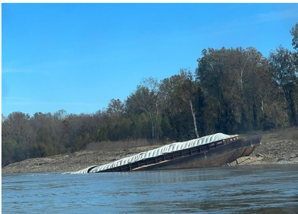
Figure 5. A barge that grounded and partially sank following the casualty. (Source: Marquette Transportation Company)
