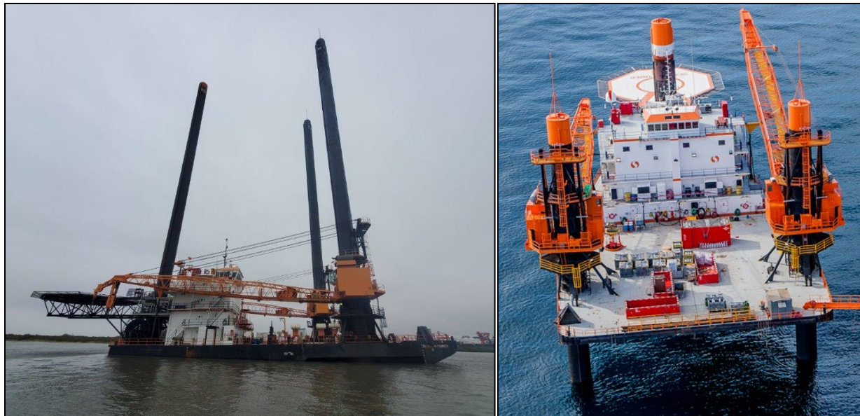
Figure 1. Precasualty photos of the SEACOR Power liftboat underway ( left ) and lifted, or “jacked up” ( right ). (Source: SEACOR Marine)
