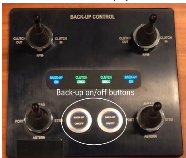
Figure 5. One of Commodore's back-up control panels, with back-up on/off buttons illuminated showing that back-up control is on. (Background source: Kongsberg Maritime)
