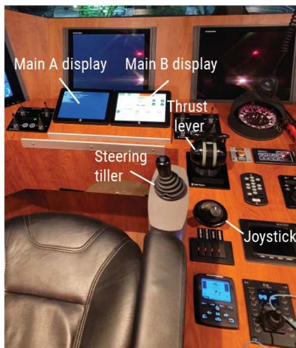
Figure 3. Commodore's main control station hand controls and water jet display screens. (Background source: US Coast Guard)
