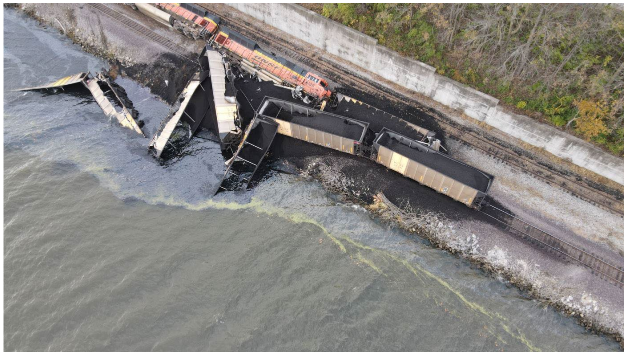
Figure 6. Aerial photo of the postcollision derailment of the two locomotives and eight hopper cars. Two additional hopper cars are submerged in the river. (Source: BNSF)
