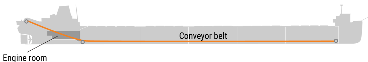
Figure 2. Simple profile of the Roger Blough showing the conveyor belt system.
