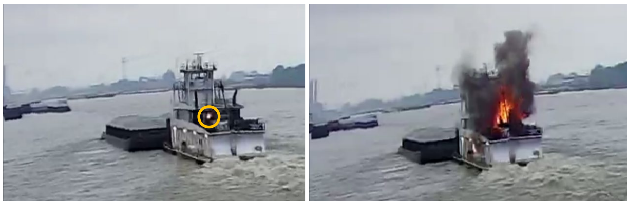
Figure 3. The Mary Lynn at 0652:40 when the first open flame, circled in yellow, was visible on the second deck port side exhaust stack (left). The Mary Lynn at 0652:45 (right). (Source: ARTCO)
