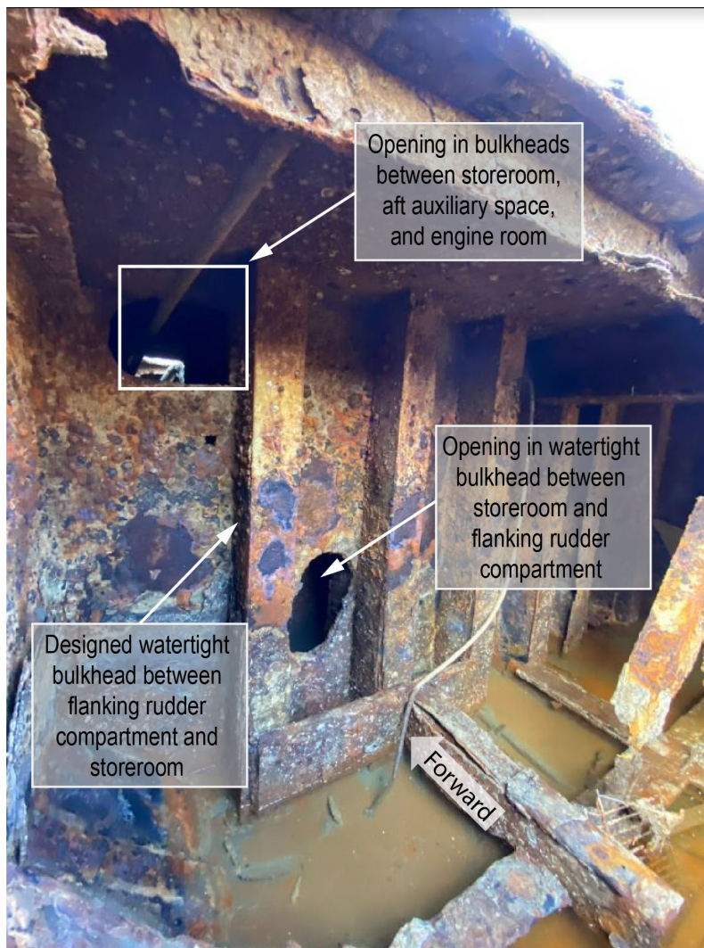
Figure 8. Flanking rudder compartment after recovery. Openings in bulkhead shown also typical of other bulkheads below the main deck separating compartments. (Source: Coast Guard)
