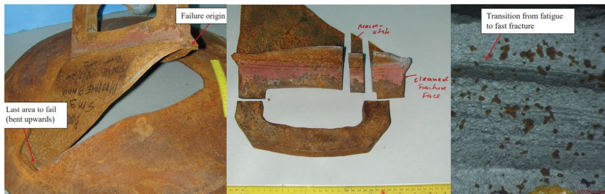
Figure 8. Simulated direction of the tear/shear failure from buoy shell (left); padeye removed, cross-section removed from weld macro-etched and fractured face cleaned (center); close-up of the fatigue crack (right). (Source: Simon Forensic, LLC)
