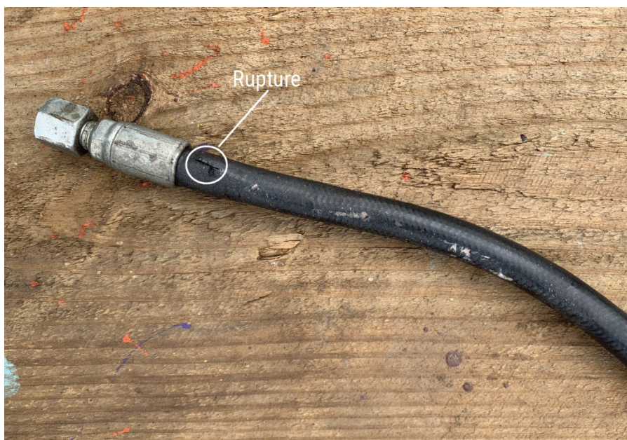
Figure 4. The ruptured port steering pump hydraulic hose, after the fire.
