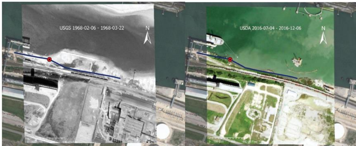
Figure 15. EPIC dock project area, 1968 and 2016, showing the extent of land loss. The blue line indicates the TX219 location, and the red circle is the approximate accident location. (Sources: US Department of Agriculture [left]; US Geological Survey [right]; photos georeferenced and overlaid on a Maxar Technologies image)
