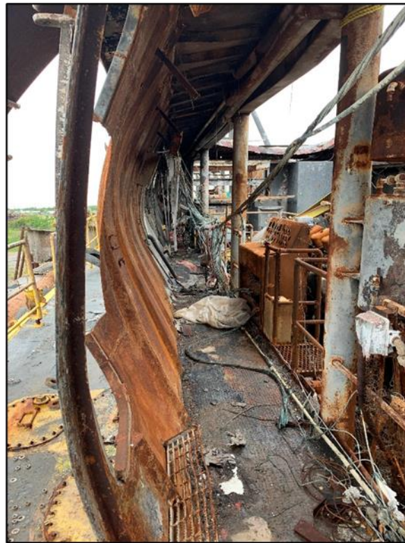
Figure 17. Post-salvage image of the Waymon Boyd engine room portside bulkhead, bowed outward.
