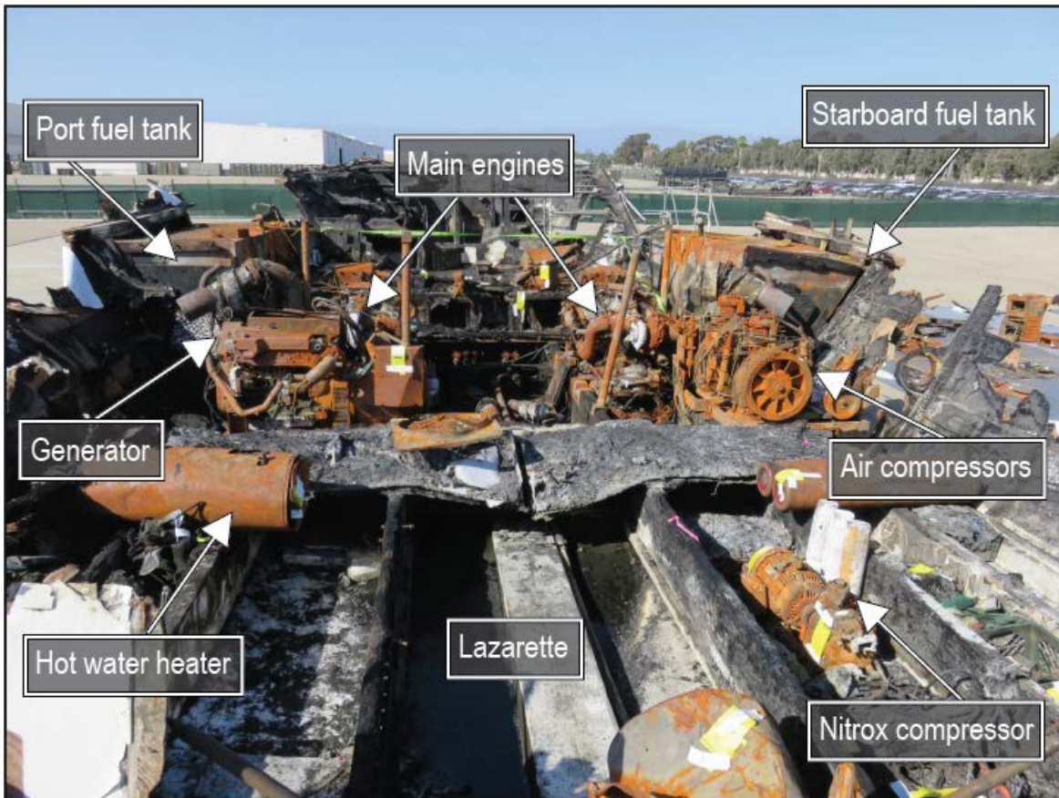
Figure 13. The salvaged hull of the Conception , looking from aft to forward, with recovered engine room and lazarette equipment placed in their original installed location (with the exception of the water heater, which was located on the starboard side).
