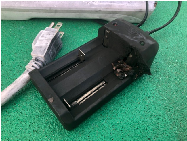
Figure 33. Photograph taken of the battery charger that caught fire on the Vision (with the batteries removed).
