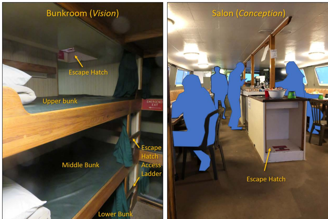
Figure 6. Photo left is the escape hatch, viewed from the bunkroom, on the Vision , a Truth Aquatics dive vessel with arrangements nearly the same as the Conception . (Source: NTSB) Photo right, taken during a previous voyage, shows the escape hatch, viewed from aft in the salon, on the Conception . (Source: J. Palmer, annotated by NTSB)
