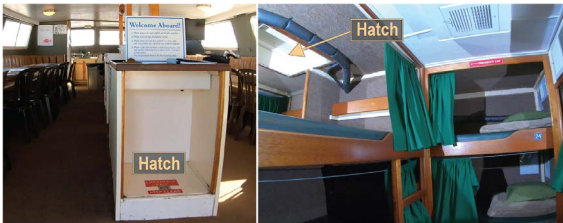
Figure 29. The Conception bunkroom escape hatch from above in the salon (left) and in the bunkroom from the port side (right). (Source: R. Clevenger [left]; Truth Aquatics [right], annotated by NTSB)
