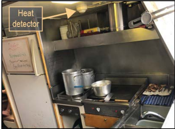
Figure 26. Photo of the galley of the Conception taken from the forward centerline window. (Source: NTSB eyewitness submission)
