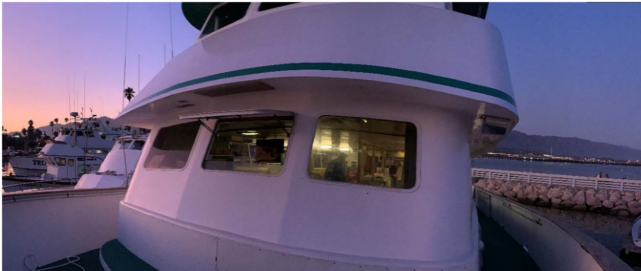
Figure 9. Preaccident photo of Conception forward salon windows. In this photo, the center window is open. However, during the accident, the window was closed and secured as the crew attempted to access the space. The port and starboard windows were not designed to be opened. (Source: T. Thompson)
