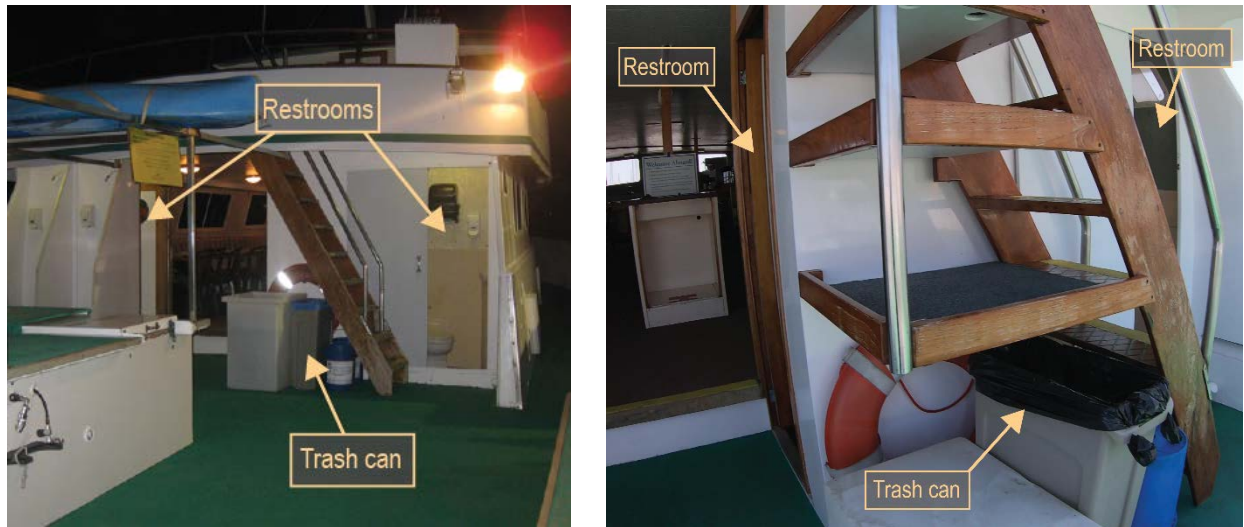
Figure 18. Left: Photo from a previous voyage of stairway to the upper deck and restrooms of the Conception . Note the regular stowage of a polyethylene trash can under the stairway aft of the salon. Right: Still image from a 2019 video taken of the stairway on board the Conception with shelving installed. (Source: M. Ryan [left], R. Clevenger [right])
