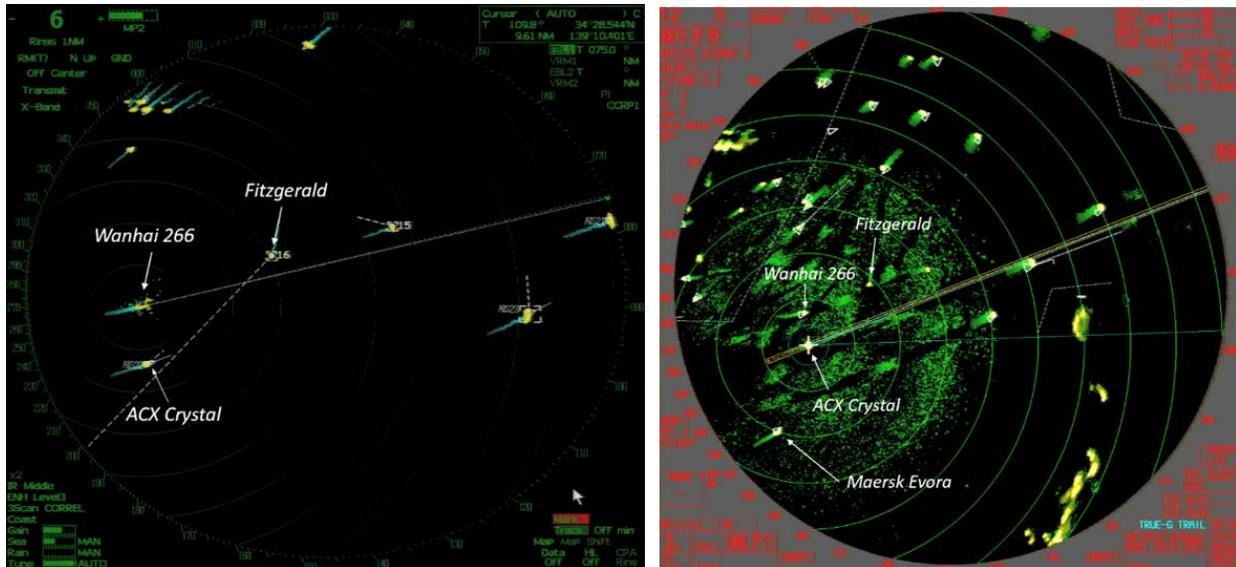
**Figure 6.** A comparison of radar screens from different vessels before the collision. Left, screen capture from the *Wan Hai 266* electronic navigation software, about 6 minutes before the collision. Right, screen capture from the *ACX Crystal* electronic navigation software (radar and ARPA), at the same time. (Vessel names have been added to screen images.)
