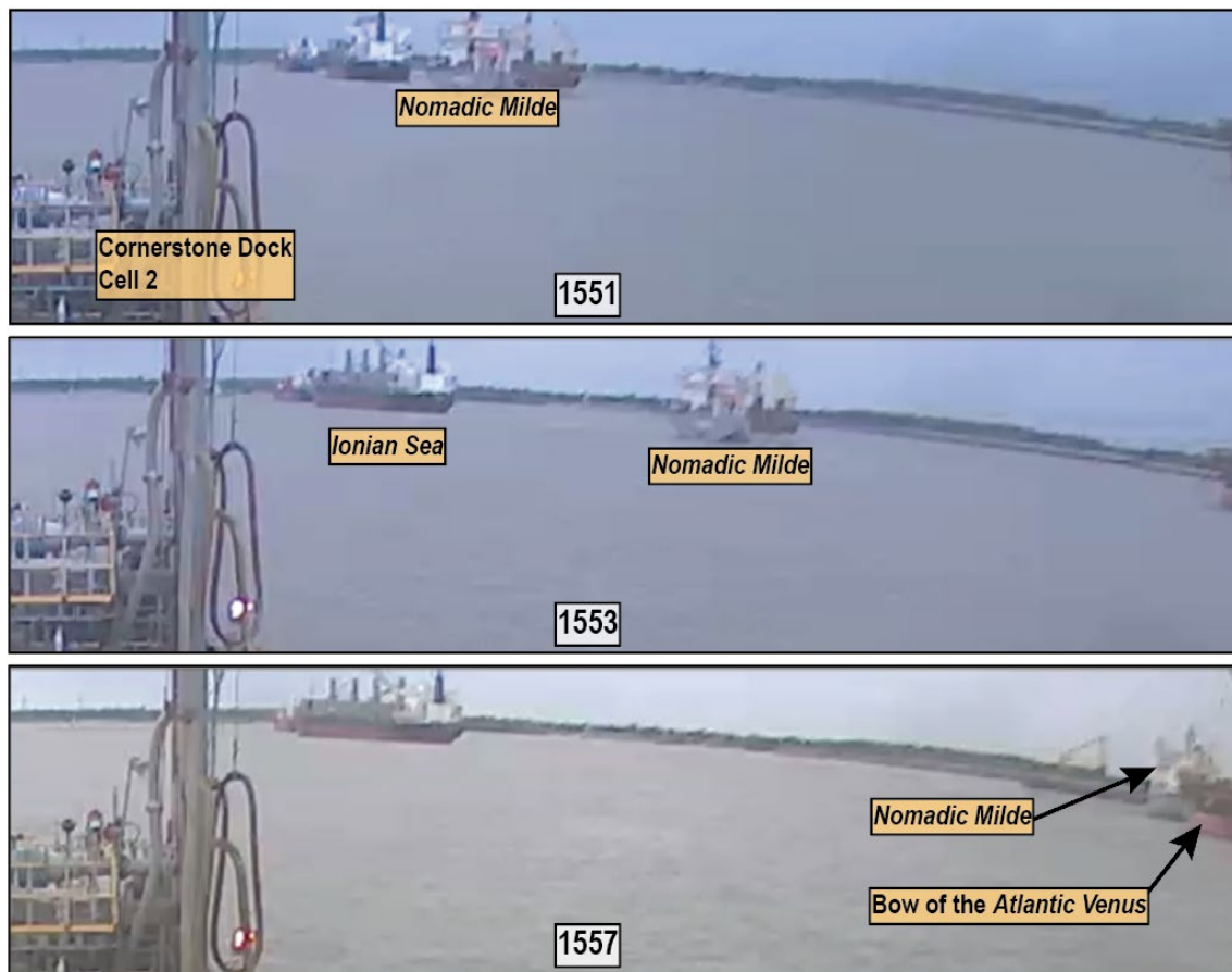
Footage from 1551, 1553, and 1557 (top to bottom) from the Cornerstone Chemical Dock showing the Nomadic Milde dragging anchor downriver towards the Atlantic Venus .
