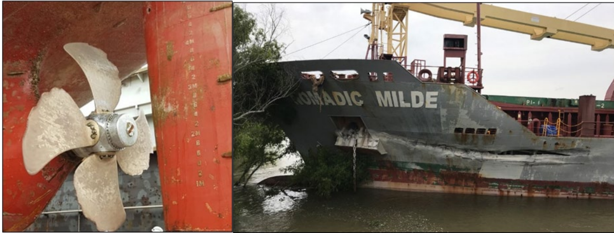
Left: Postaccident damage to the Nomadic Milde 's propeller. (Source: Intership Navigation Co. Ltd) Right: Nomadic Milde on the right descending bank at the Cornerstone Dock showing a gash in the hull aft of the port anchor pocket. (Source: US Coast Guard)
