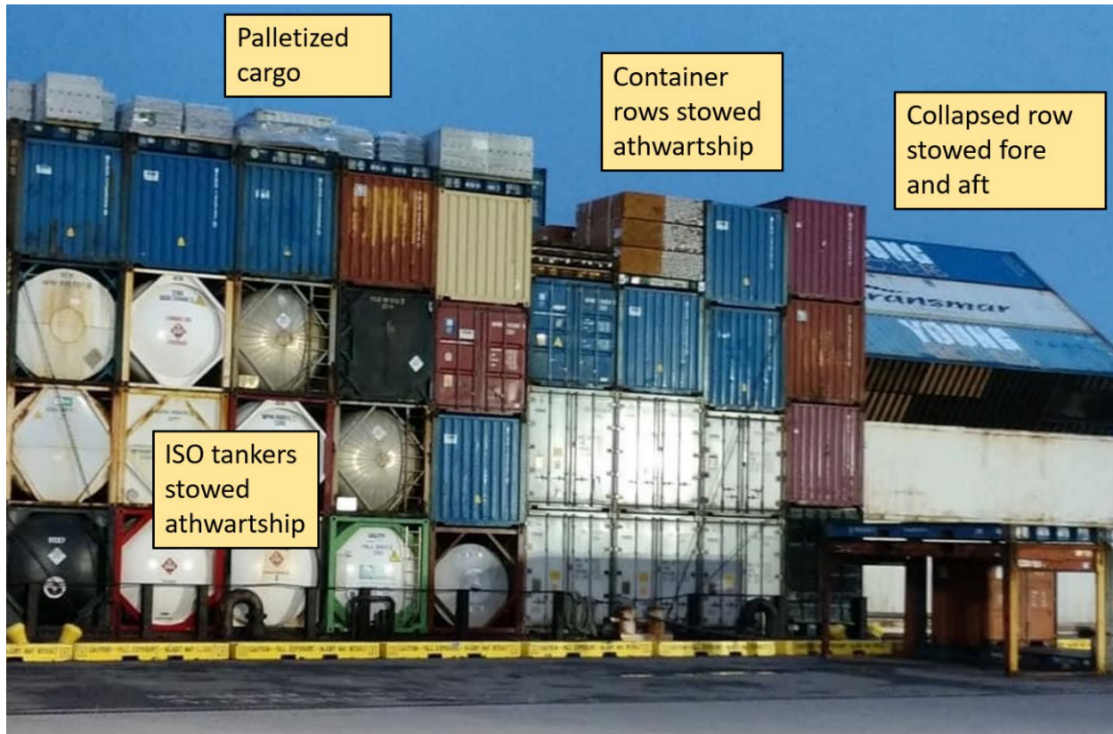
Cargo on the Ho'omaka Hou upon arrival to Hilo at the end of the accident voyage.
