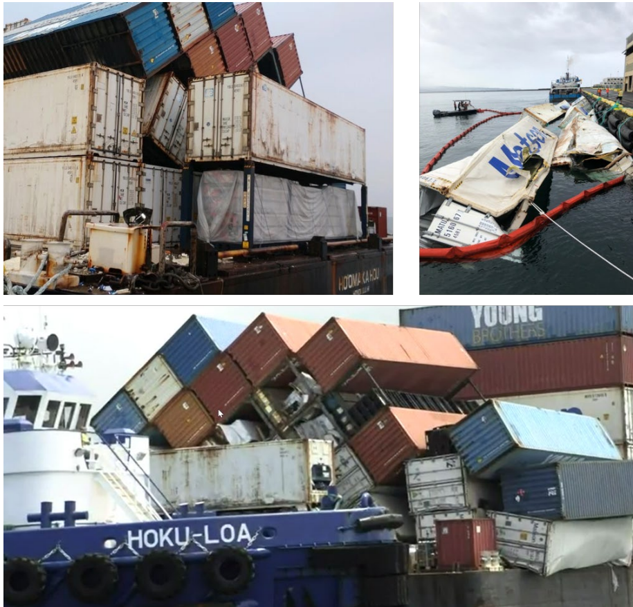
Clockwise, from top left: The collapsed row of containers on the barge in Hilo; salvaged containers, pier side in Hilo; and the collapsed row of containers, from the starboard quarter of the Ho'omaka Hou . (Source: Coast Guard)
