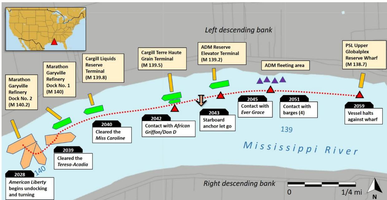
From where the *American Liberty* was moored, there were five wharfs on the left descending bank downriver. All vessels were moored starboard-side-to, bow pointed upriver. Shown is the vessel’s AIS track (red dots) getting underway, turning counterclockwise, moving bow first downriver, and contacting vessels and wharfs along the left descending bank, as indicated by the red triangles. Not to scale. (Background Source: Google Maps)
